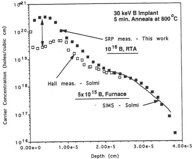
Fig. 3 Comparison between B activation after 800 °C, 5 min RTA and furnace anneals for high dose B implants at 30 keV.
