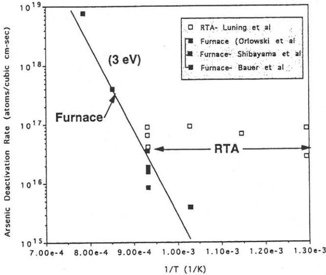
Fig. 2 Observation of optically enhanced As deactivation rates at temperatures below 850 °C.
