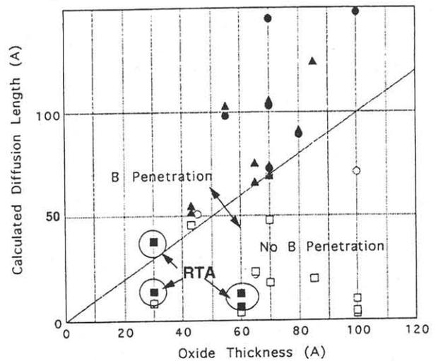
Fig. 4. Calculated vs measured B penetration lengths in oxides. B penetration through oxides: nitrided oxide (●) and SiO<sub>2</sub> (▲); no penetration: nitrided oxide (○) and SiO<sub>2</sub> (△). RTA anneals result in anomalous penetration.
