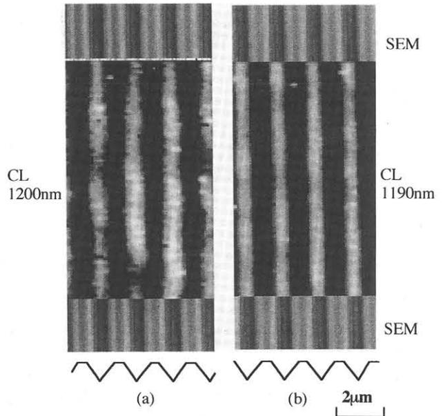
Fig.2 CL and SEM images of InGaAs quantum wire structures. The InGaAs quantum wire layers of (a) and (b) were grown without and with atomic hydrogen, respectively.
