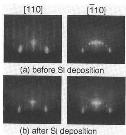
Fig.1. RHEED patterns before and after Si deposition.
