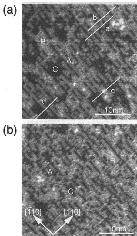
Fig.3. STM images taken after the Si deposition ((a):1/8 ML in the As pressure of  $0.9 \times 10^{-8}$  Torr, (b)1/4 ML in  $1.5 \times 10^{-8}$  Torr).
