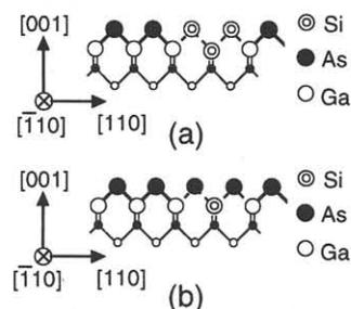
Fig.5. Possible models for the microscopic structure of the trench filling Region B.
