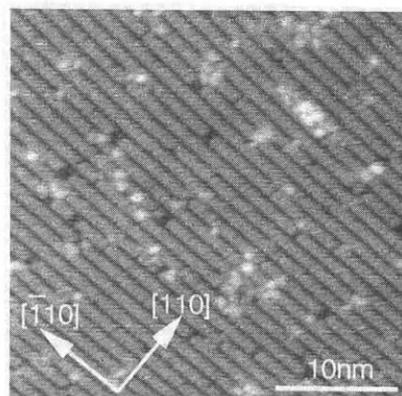
Fig.2. A typical filled state STM image taken on the initial GaAs(2x4)  $\beta$ -phase surface.
