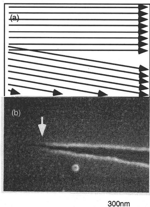
Fig.4. Sharp angle resist pattern .
