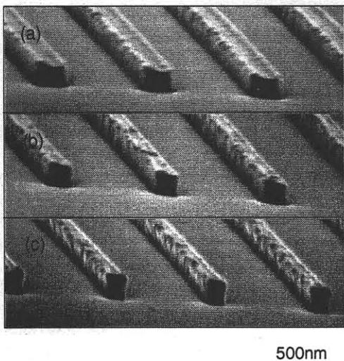
Fig. 3 Cross-sectional SEM pictures of the resist patterns. Exposure dose of (a) 105nC/cm, (b) 28nC/cm, (c) 13nC/cm.
