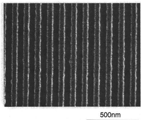
Fig. 1 SEM picture of line and space resist pattern at 40nm.
