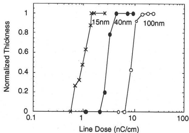
Fig.2 Sensitivity curve of MRS using AFM.
