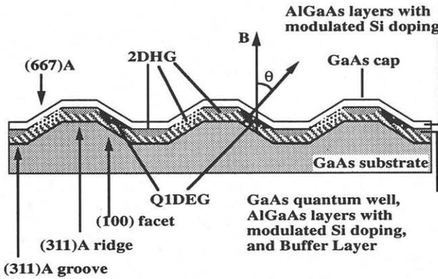
Fig. 1 Cross sectional schematic diagram of the device structure.
