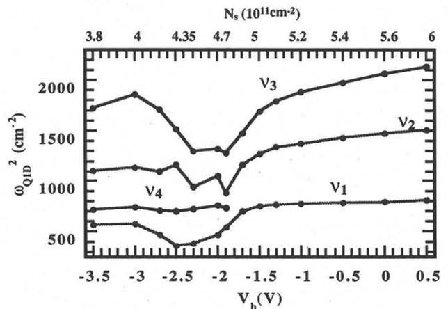
Fig. 3 Square of the resonant frequency  $(\omega_{Q1D})^2$  vs.  $N_s$  and  $V_h$ . For  $V_h > -1.9$  V the plot clearly shows an increasing rate of change of  $(\omega_{Q1D})^2$  for decreasing  $V_h$  while the carrier density decreases linearly. This is explained by increase in non-parabolicity of the confining potential. This is also supported by the appearance of the new mode  $v_4$  for  $V_h < -1.9$  V.
