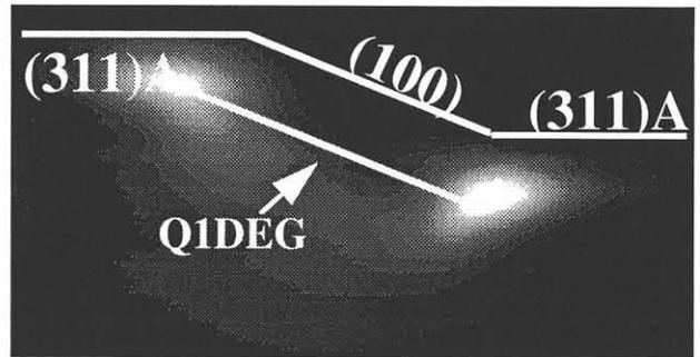
Fig. 2 EBIC measured at  $V_h = -1.0$  V. The brighter regions are associated with higher electric field. The picture shows a non-symmetric profile along the confinement direction. The strong non-parabolicity which results is responsible for the new mode  $v_4$  in the FIR spectra.
