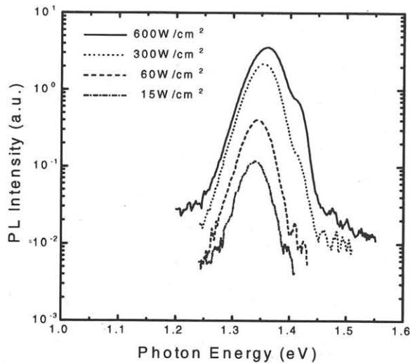
**Fig. 3.** 77K PL of 1.7 ML InAs/GaAs SADs excited by 514.5nm laser at different excitation intensities. Both InAs dots and GaAs cap layer were grown at 450°C.
