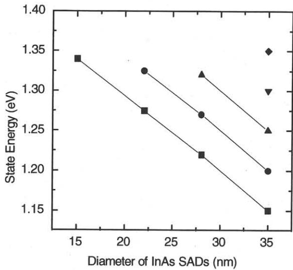
**Fig. 2.** Peak positions of the Gaussian components in the 77K PL spectra of the four samples with different dot sizes.
