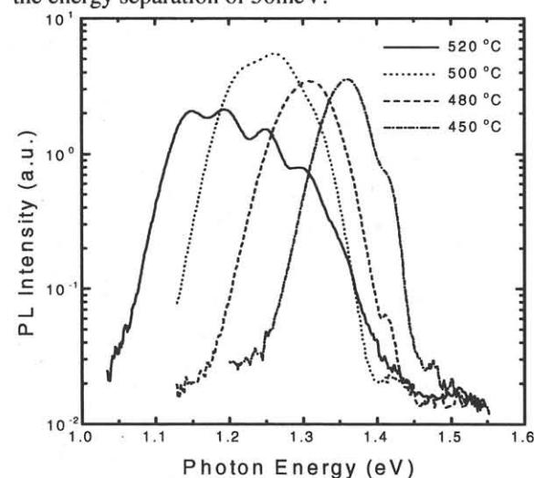
**Fig. 1.** 77K PL of 1.7 ML InAs/GaAs SADs excited by 514.5nm laser at 600W/cm<sup>2</sup>. InAs were deposited at 520°C, 500°C, 480°C, 450°C, respectively and all of them were capped by GaAs at 450°C.
