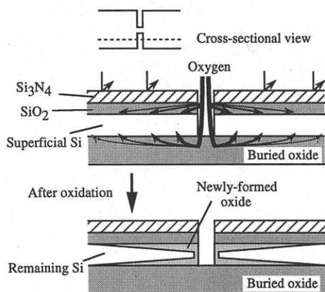
Fig. 4 Schematic diagram of SiN-masked pattern-dependent oxidation. The Si layer away from the pattern-edge remains thick.
