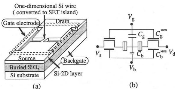
Fig. 1 (a) Schematic diagram of a Si SET. (b) The equivalent circuit.
