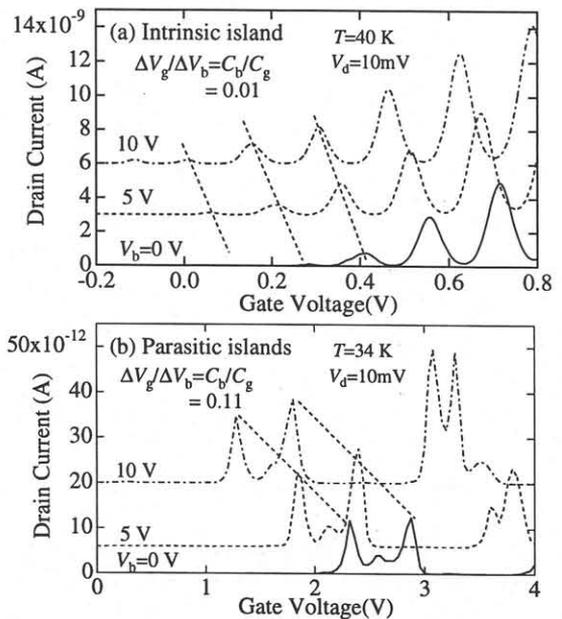
Fig. 2  $I$ - $V_g$  characteristics for (a) Si-SET with a relatively thick Si layer and (b) another SET with a thin Si layer. The curves are vertically offset for clarity. Note the different voltage scales for (a) and (b).
