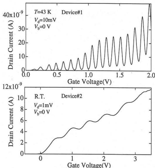
Fig. 5  $I$ - $V_g$  characteristics of Si-SETs fabricated by SiN-masked pattern-dependent oxidation. (a) The device with relatively thick Si and (b) the other device with a thin Si layer.
