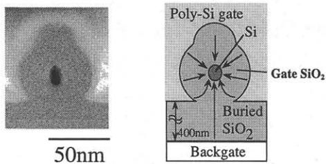
Fig. 3 Cross-sectional TEM of the Si wire and its schematic diagram.
