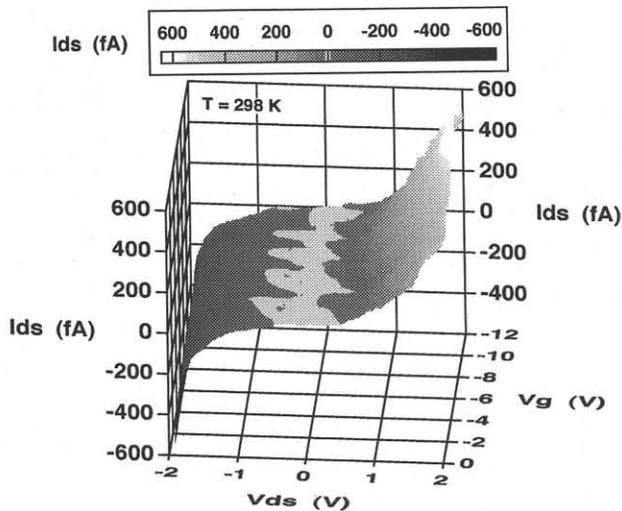
Figure 2. Drain current-drain voltage characteristics with various side-gate voltages at room temperature ( $T = 298$  K). Drain current with  $\pm 2$  fA is colored as white.
