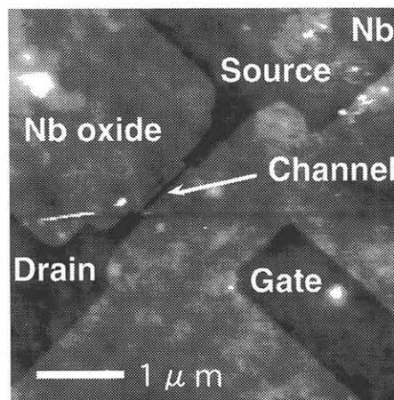
Figure 1. AFM image of side-gate SET. Tunnel junctions are not well resolved in this magnitude.
