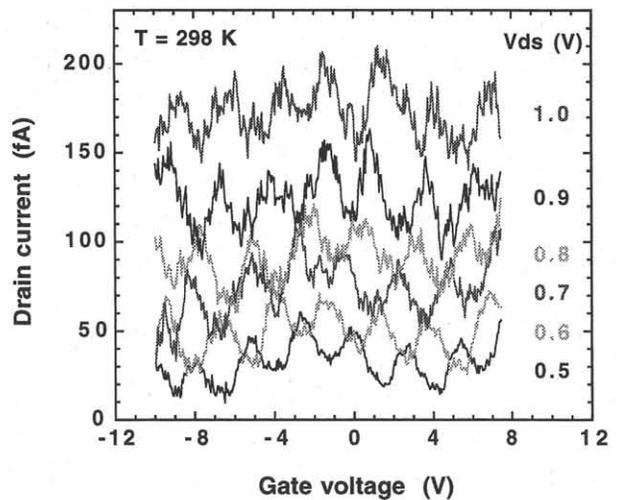
Figure 3. Drain current-gate voltage characteristics with various drain voltages at room temperature ( $T = 298$  K).
