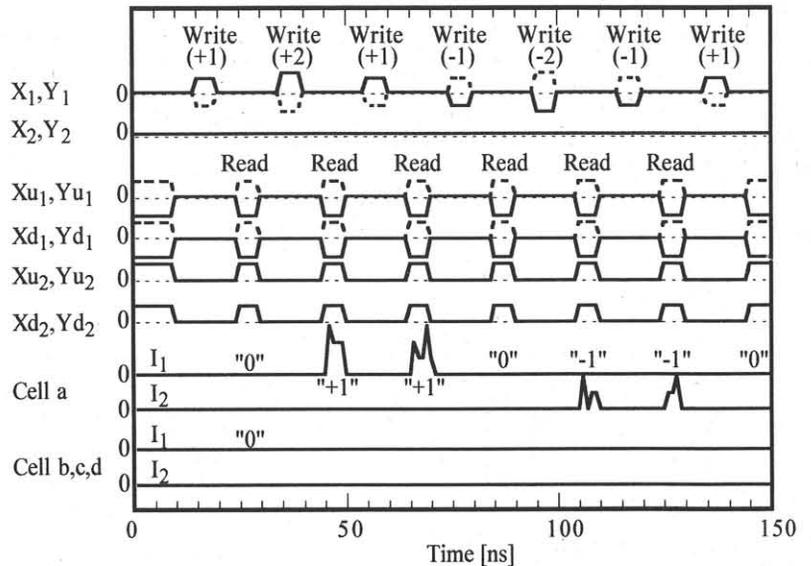
**Fig. 3** Simulation of data writing and reading performances of the memory array shown in Fig. 2 under a room temperature condition. The thick lines show writing and reading voltages and data reading currents I<sub>1</sub> and I<sub>2</sub> for each memory cell.
