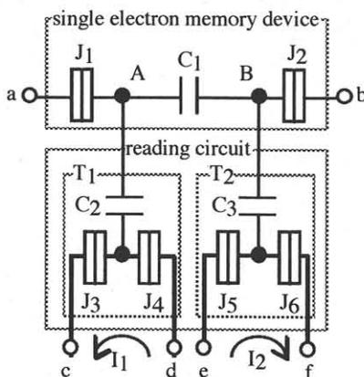
Fig.1 Schematic of a memory cell constructed with a single electron memory device and a reading circuit.
