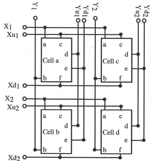
Fig. 2 Schematic of the memory array circuit constructed with the memory cells which are shown in Fig. 1.
