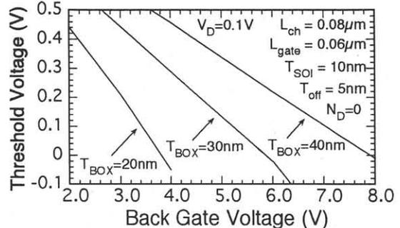
Fig.7  $V_{th}$  dependence on  $V_{bg}$ . The result indicates that a thin  $T_{BOX}$  is suitable for decreasing  $V_{bg}$ , and that a thick  $T_{BOX}$ , where the  $V_{th}$  weakly depends on  $V_{bg}$ , is suitable for reducing the body effect.
