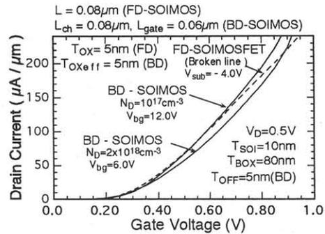
Fig.6 Comparison on the ON current at saturation region. The drain current of a BD-SOIMOS having low body concentration is comparable with the fully depleted SOI-MOSFET having the intrinsic body( broken line). The current for  $V_g>0.6V$  is increased by the lateral BJT current.
