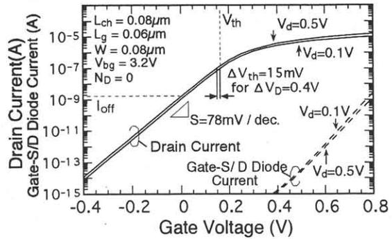
Fig.4 The subthreshold characteristics for BD-SOIMOS. The gate-S/D current corresponds to the base current of BJT. The band to band tunneling is not included in the simulation.
