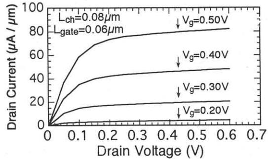
Fig.5  $I_D$ - $V_D$  characteristics for BD-SOIMOS.
