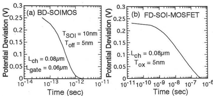
Fig3 Transient behaviors after excess holes are induced. (a) for BD-SOIMOS, (b) for a usual fully depleted SOI-MOSFET having the same channel length as (a). In (b), the potential deviation remains more than 10nsec.
