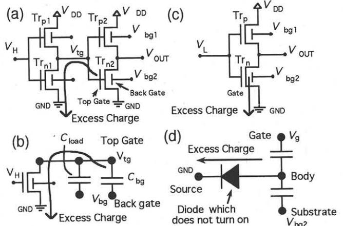
Fig.2 Excess charge pass. (a) BD-SOIMOS, (b) Its equivalent circuit, (c) Usual SOI-MOS and (d) Its equivalent circuit.
