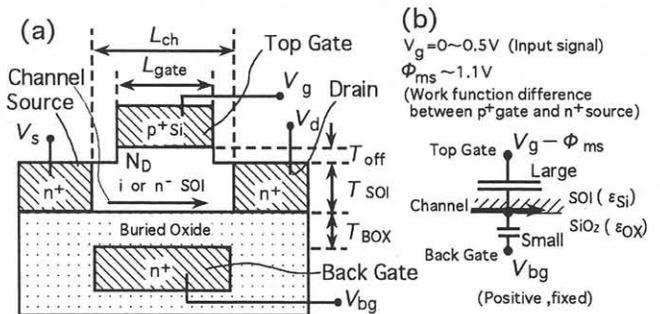
Fig.1 (a) The device structure of BD-SOIMOS.(b) The relation between the top gate and the back gate capacitance.
