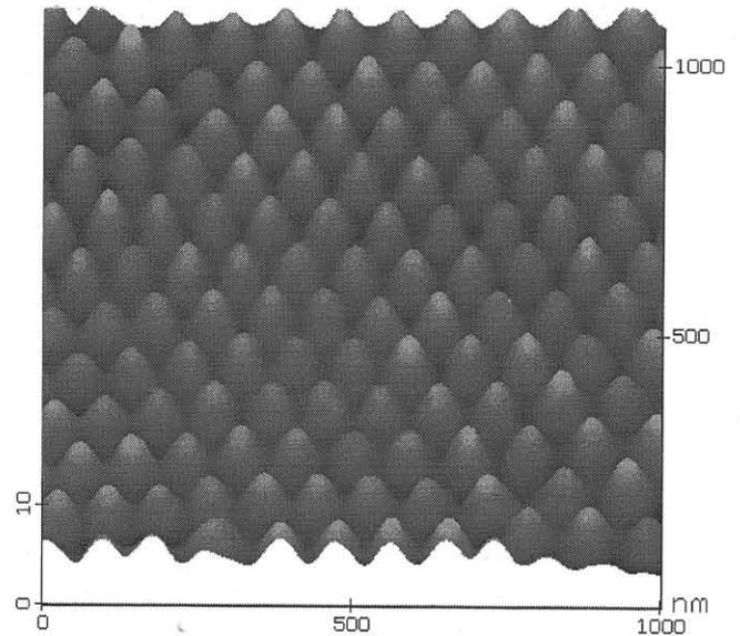
Figure 2: Raw atomic force micrograph of the surface features in a thin aluminum film produced by electropolishing. This can be used to realize a two dimensional array of metallic islands of  $\sim 30$  nm diameter.
