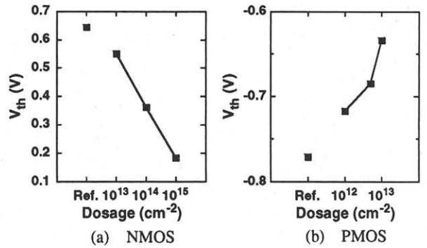
Fig. 1.  $V_{th}$  adjustment scheme by using  $H^+$  implantation.
