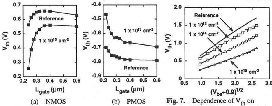
Fig. 6. Dependence of threshold voltage on gate length (100-keV implantation,  $V_{th}$  at  $V_d=2.5 V$ ,  $I_d=0.2 \mu A$ ).
