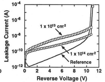
Fig. 8. Junction leakage current of  $500 \mu m \times 500 \mu m$   $N^+/P$  junction (100-keV implantation).
