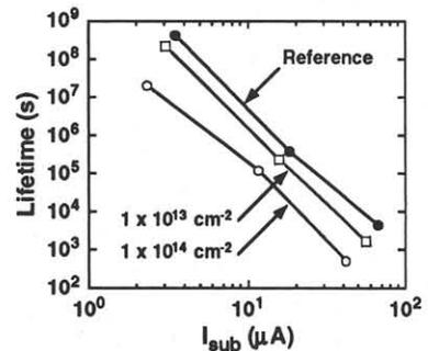
Fig. 11. Hot carrier lifetime of MOSFET under drain avalanche hot carrier injection (lifetime was defined as the time for 10 % degradation of  $I_d$ , stressed at  $V_g$  of  $I_{submax}$ ,  $I_d$  was measured at  $V_d=V_g=2.5 V$ ).
