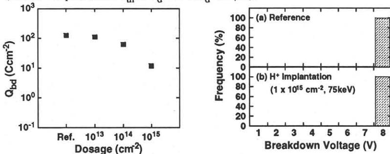
Fig. 9. Dependence of charge-to-breakdown of MOSFET on hydrogen ion dosage (75-keV implantation, stress current  $=0.5 A cm^{-2}$ , at 300 K).
