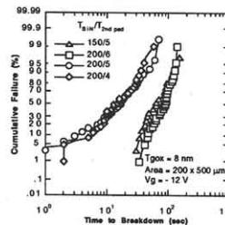
Fig. 2 TDDDB data with various process conditions.
