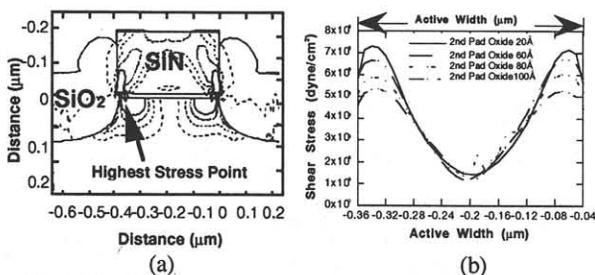
Fig. 7 RPSL stress simulation results in (a) 2-D and (b) 1-D. TSUPREM-IV was used.
