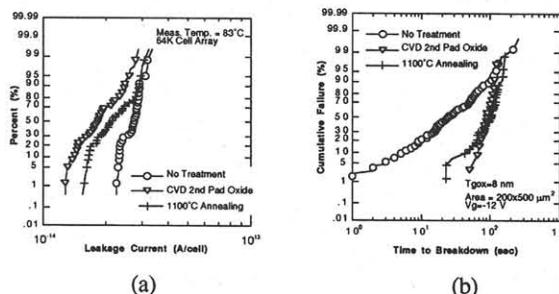
Fig. 9 Cell junction leakage current data with the stress released RPSL isolation. Fig. 10 TDDB data of the stress released RPSL isolation.
