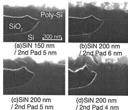
Fig. 4 Final isolation profiles with various process conditions and gate oxide thinning in each case.
