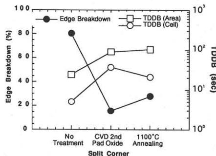
Fig. 11 Edge breakdown vs. TDDB time in the stress released RPSL isolations.
