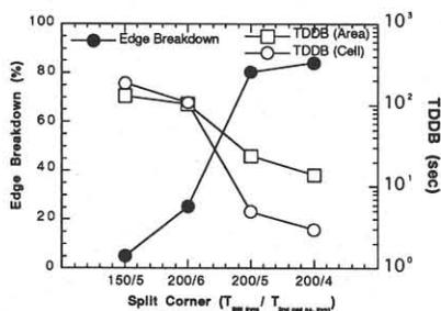
Fig. 6 Relation of the breakdown position with TDDB time.
