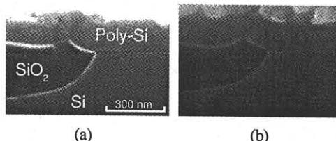
Fig.8 SEM micrographs of the stress released RPSL isolation. (a) 1100°C annealing and (b) 5 nm CVD 2nd pad oxide.
