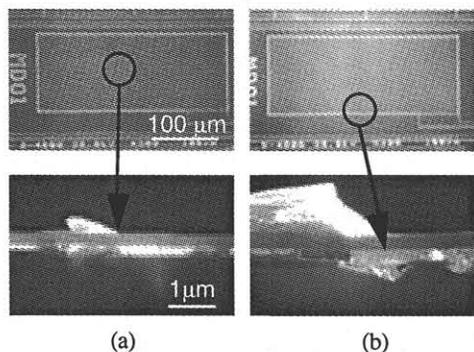
Fig. 5 SEM micrographs of the gate oxide breakdown. (a) Center Breakdown. (b) Edge Breakdown.
