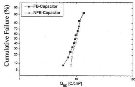
Fig. 6 The Gate oxide charge-to-breakdown at  $J=-100\text{mA}/\text{cm}^2$  between field butted and non field butted capacitor pattern.
