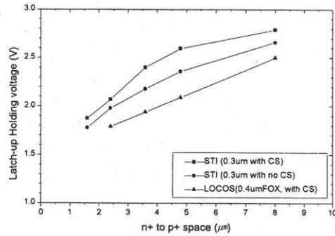
Fig. 4 The latchup holding voltage vs. n+/p+ spacing
