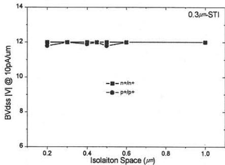
Fig. 3 The n+/n+ or p+/p+ isolation punch-through voltage characteristics
