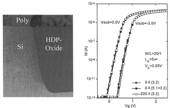
Fig.1 (a) TEM picture of finished STI profile with S/W oxide of 68 $\text{\AA}$  and (b) subthreshold  $I_D$ - $V_G$  characteristics
