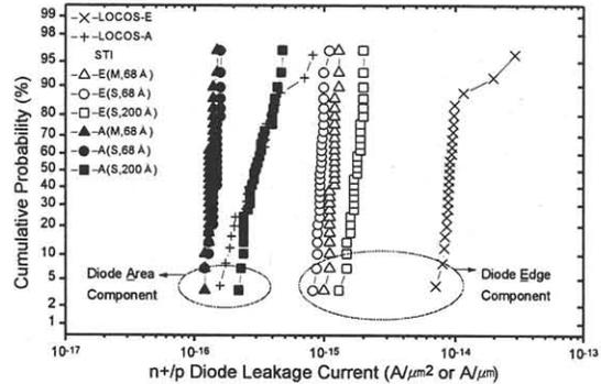
Fig. 5 n+/p diode leakage current with split conditions at  $V_R=4.0\text{V}$ , compared to LOCOS ( $1900\text{\AA}/100\text{\AA}$ : Nit/oxide): E (Edge), A (Area), S (Single D/S, 3.2), M (Multi D/S, 8.0 + 5.1+3.2)
