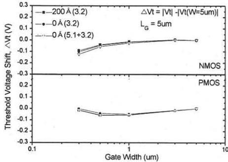
Fig. 2 The threshold voltage shifts,  $\Delta V_T$ , between  $W$  and  $W=5\mu\text{m}$  for both nMOS with INWE and pMOS with NWE.
