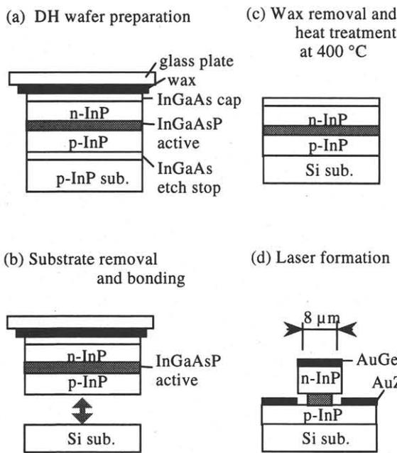
Fig. 1: Fabrication process of InGaAsP edge-emitting lasers on Si by wafer bonding.
