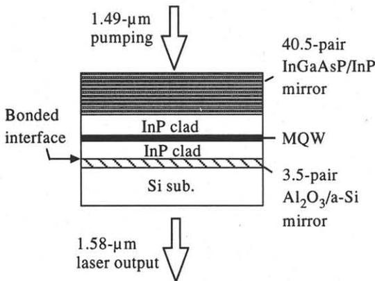
Fig. 3: Schematic structure of InGaAsP surface-emitting lasers on Si fabricated by wafer bonding.
