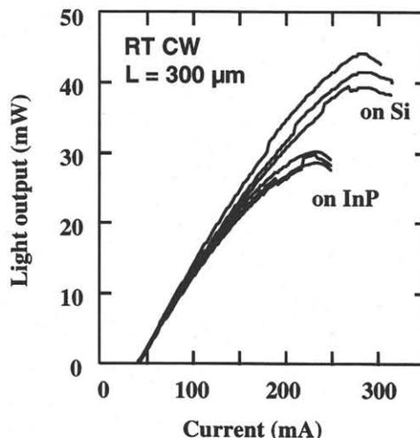
Fig. 2: Light-current characteristics of the edge-emitting lasers under room-temperature CW excitation.
