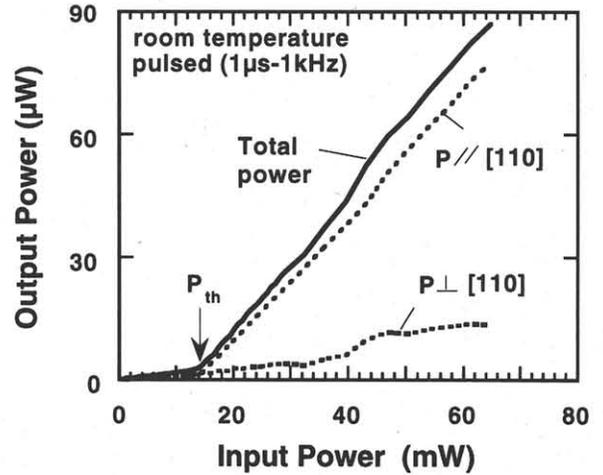
Fig. 4: Light output versus input power characteristics at room temperature.
