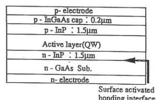
Figure 1. Schematic diagram of a 1.3  $\mu\text{m}$  InGaAsP laser on a GaAs substrate using the surface activated wafer direct bonding method.
