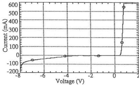
Figure 3. Current -voltage characteristic of the laser fabricated on GaAs substrate using surface activated wafer direct bonding.
