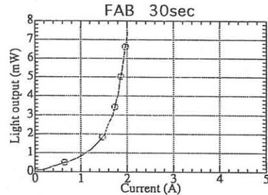
Figure 5. Light-current characteristic of the laser fabricated on GaAs substrate using using surface activated wafer direct bonding.
