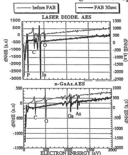
Figure 2. Auger Electron Spectra(AES) of LD and GaAs substrate surfaces before and after 30 seconds Ar FAB cleaning.
