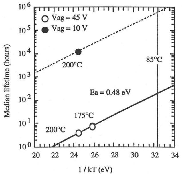
Fig. 5 Arrhenius plot of median lifetime versus temperature with aging voltage as a parameter.
