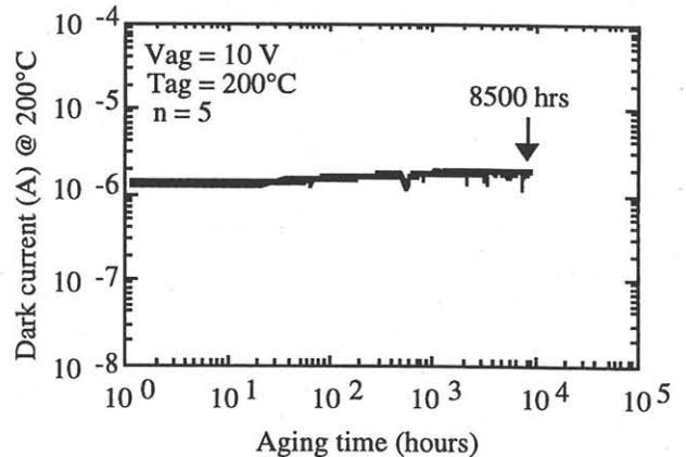
Fig. 2. Long-term aging test at 200°C and a bias voltage of 10 V. The vertical axis shows the in situ dark current.
