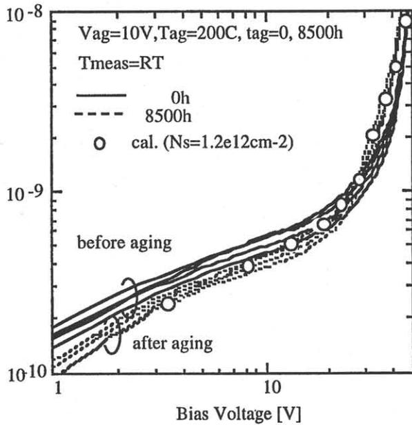
Fig. 3 I-V characteristics of WG-PDs before and after 8500-hr aging at 200 °C and calculated degradation by carrier injection model.
