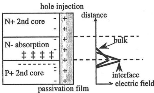
Fig. 4 Carrier injection model
