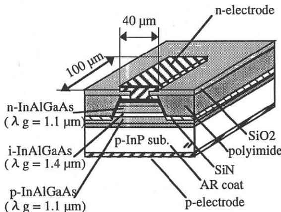
Fig. 1. Schematic structure of the InGaAlAs mesa-waveguide photodiode with a double-core structure.
