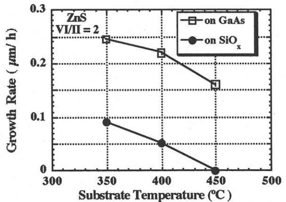
Fig. 1 Growth temperature dependence of ZnS. Selective growth was observed at 450°C.
