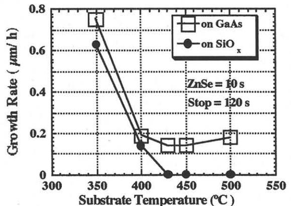
Fig. 3 Growth temperature dependence of ZnSe using periodic supply epitaxy. Selective growth was observed at 450°C.
