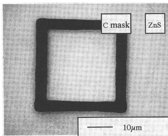
Fig.6 SEM picture of ZnS selective growth using C mask. Good selectivity was observed at 390°C.
