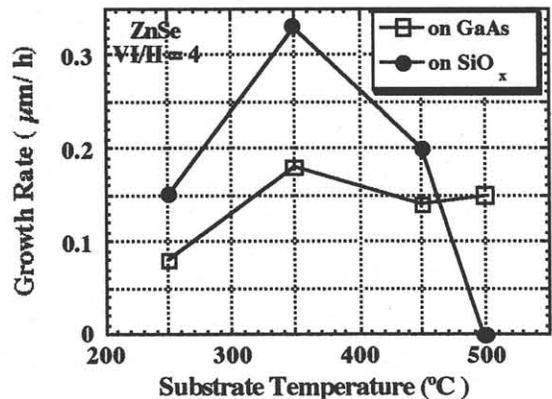
Fig. 2 Growth temperature dependence of ZnSe. Selective growth was observed at 500°C.
