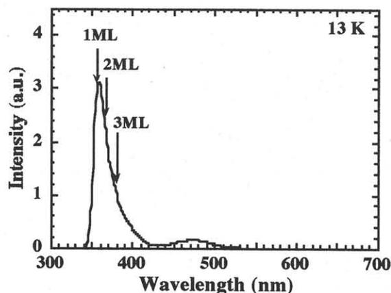
Fig.5 Photoluminescence spectrum of ZnSe/ZnS SQW at 13K. Arrows shows the optical transition wavelength calculated for the ZnSe well width of 1, 2, and 3 monolayer. The bright band edge emission from the ZnSe well was observed.
