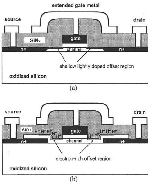
Fig. 1 Cross-section of gate-overlapped lightly doped drain (GO-LDD) TFTs (a) with ion shower doping (b) with *in-situ* doped source and drain.
