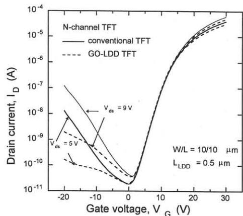
Fig. 2 The I<sub>D</sub>-V<sub>G</sub> curves of the new GO-LDD TFTs with 270 Å-thick buffer oxide by employing the ion shower doping. The thickness of SiN<sub>x</sub> interlayer is 6000 Å.
