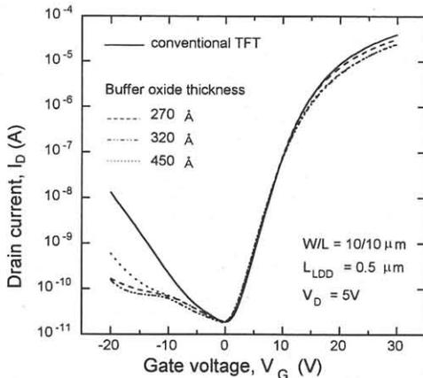
Fig. 3 The  $I_D$ - $V_G$  curves of the new GO-LDD TFTs with 6000 Å-thick  $\text{SiN}_x$  interlayer as a function of buffer oxide thickness.
