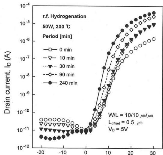
Fig. 5 The  $I_D$ - $V_G$  curves of the GO-LDD TFT with *in-situ* doped source and drain as a function of hydrogenation period.
