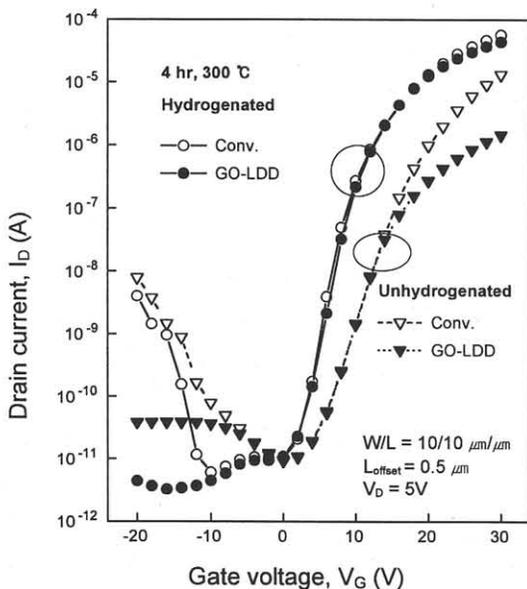
Fig. 4 The  $I_D$ - $V_G$  curves of conventional non-offset TFT and GO-LDD TFT with *in-situ* doped source and drain before and after 4 h hydrogenation.
