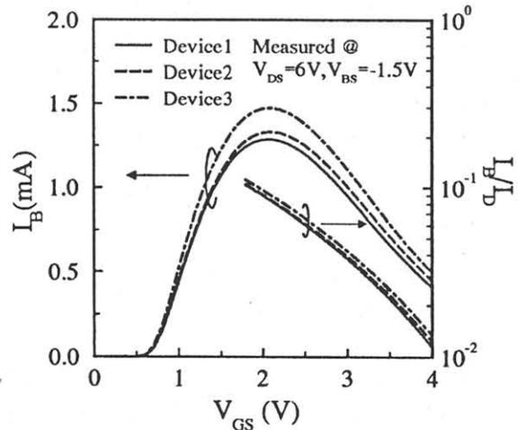
Fig. 2 Measured substrate currents and the impact ionization rate ( $I_B/I_D$ ) for three devices.
