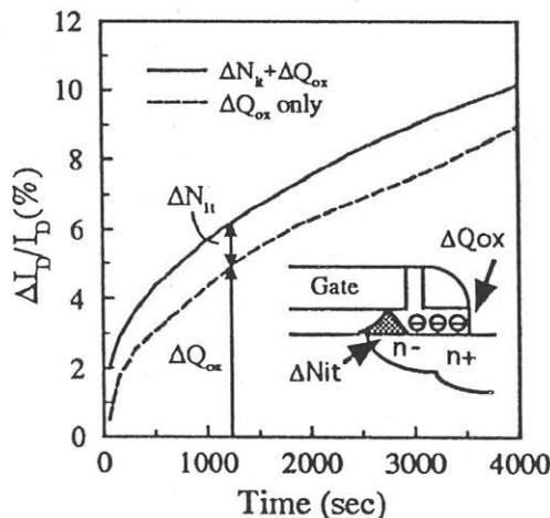
Fig. 7 Individual contribution of the interface state and oxide trap charge to the drain current degradation for Device 2.
