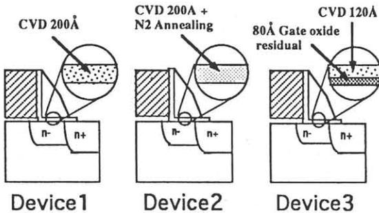
Fig. 1 Device structures used in this study. All of three devices have different post-oxides under the nitride spacer.
