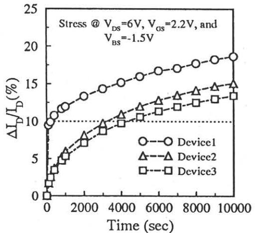
Fig. 3 Measured drain current degradation versus stress time for three devices under maximum substrate current stress.
