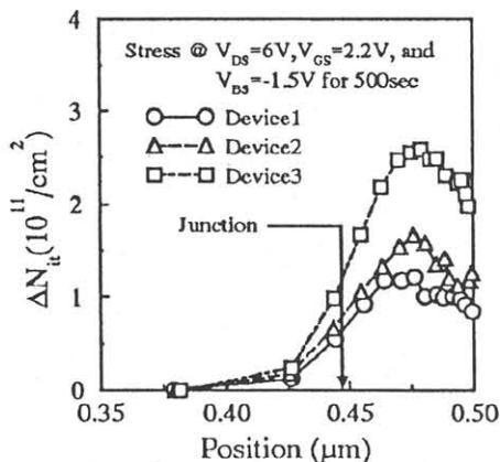
Fig. 4 Calculated lateral distribution of the interface states for three devices.
