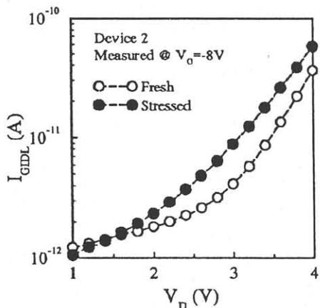
Fig. 5 Measured fresh and stressed GIDL currents of Device 2.
