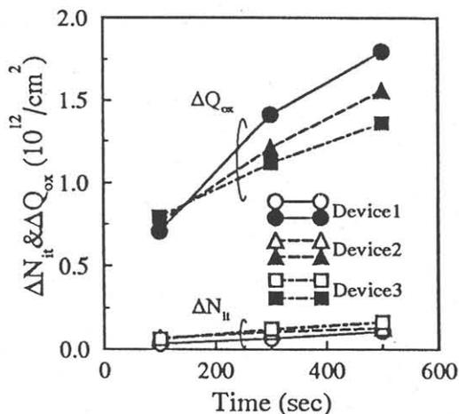
Fig. 6 Calculated total amount of oxide damages (interface state and oxide charge) for three devices.
