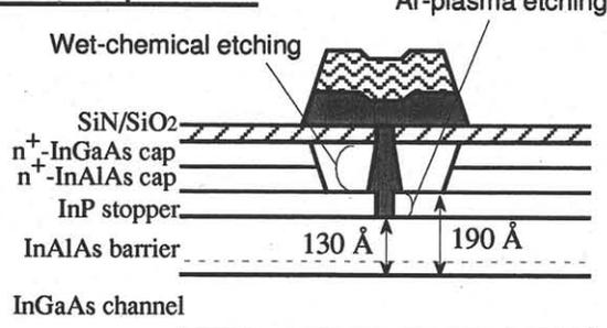
Fig. 1. Schematic cross section of gate structure of conventional and *two-step recess* process. In two-step recess process, InP stopper layer is removed by Ar-plasma dry etching to avoid side-etching.
