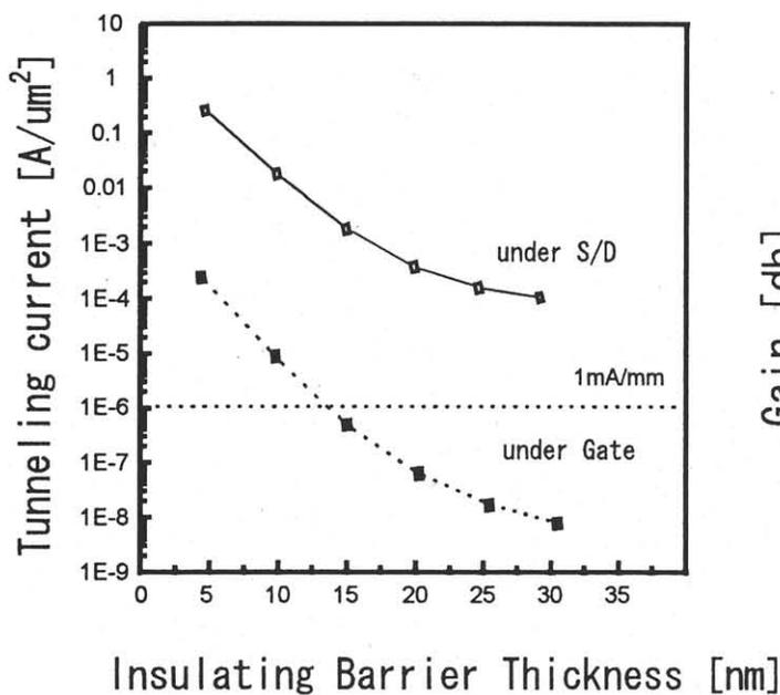
Fig. 2 Dependence of tunneling current on barrier thickness
