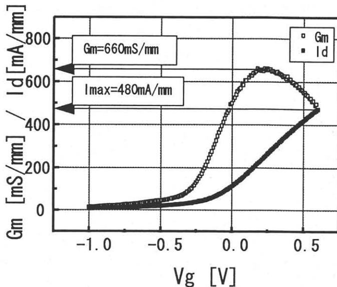
Fig. 3 DC characteristics of 0.2um gate DC-HFET
