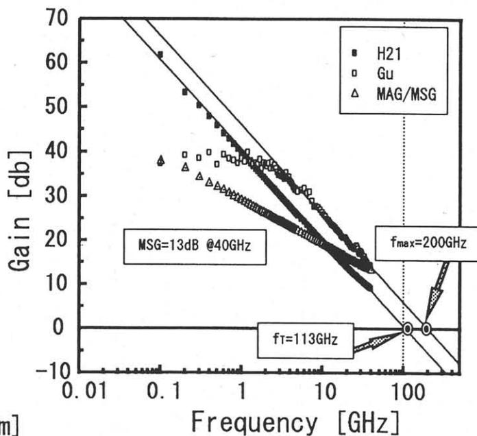
Fig. 4 RF characteristics of 0.2um gate DC-HFET
