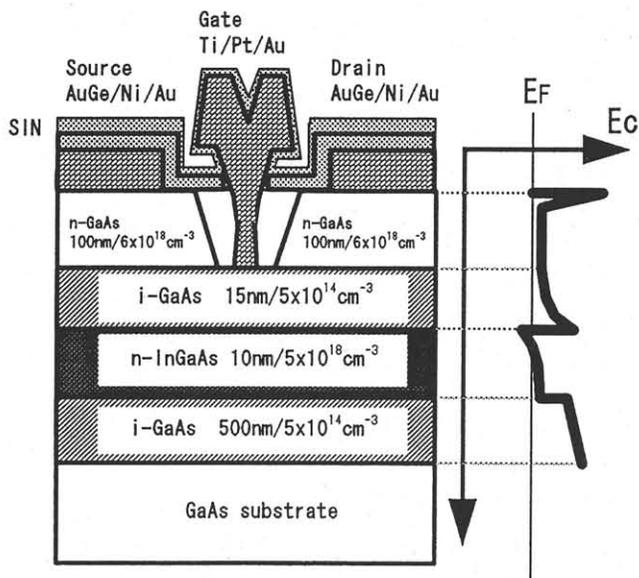
Fig. 1 Cross-section and Energy band diagram of DC-HFET
