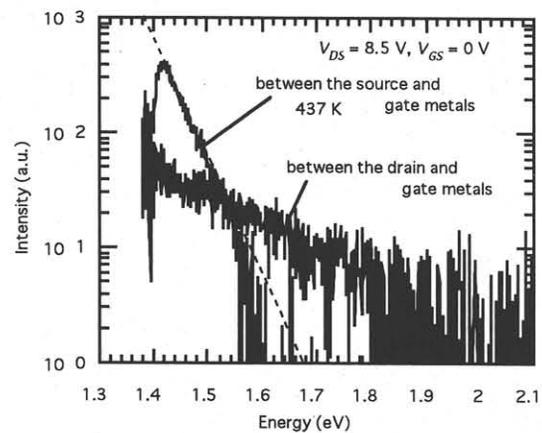
Fig. 5 Micro-EL spectra for regions between the source and gate metals, and between the gate and drain metals at  $V_{DS} = 8.5 \text{ V}$  and  $V_{GS} = 0 \text{ V}$ .
