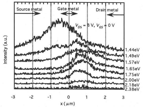
Fig. 3 The EL spatial distribution for various luminescence energies at  $V_{DS} = 8 \text{ V}$  and  $V_{GS} = 0 \text{ V}$ . The measurement was performed in the configuration that the source, gate, and drain metals cover regions  $x < -1.5 \mu\text{m}$ ,  $-0.5 \mu\text{m} < x < 0.5 \mu\text{m}$  and  $2 \mu\text{m} < x$ , respectively.
