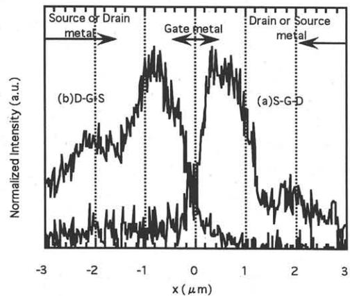
Fig. 4 The spatial distribution of 2.0 eV luminescence measured for two different arrangements that the source, gate, and drain metals cover regions (a)  $x < -1.5 \mu\text{m}$ ,  $-0.5 \mu\text{m} < x < 0.5 \mu\text{m}$  and  $2 \mu\text{m} < x$ , and (b)  $2 \mu\text{m} < x$ ,  $-0.5 \mu\text{m} < x < 0.5 \mu\text{m}$  and  $x < -1.5 \mu\text{m}$ , respectively.
