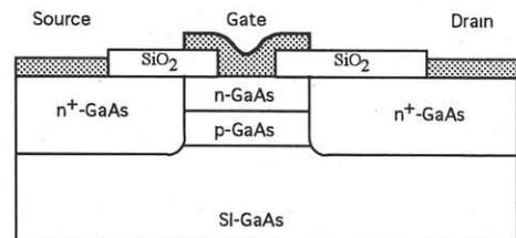
Fig. 1 The schematic cross section of the measured GaAs MESFETs.
