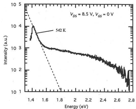
Fig. 2 The EL spectrum at  $V_{DS} = 8.5$  V and  $V_{GS} = 0$  V.
