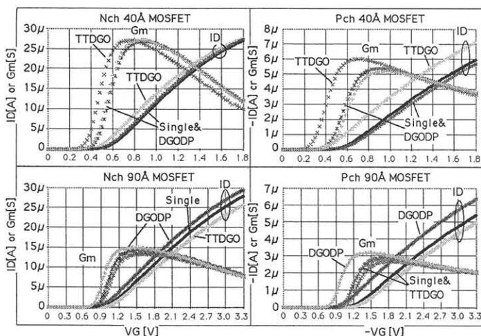
Fig 3. MOSFET characteristics (W/L=18μm/18μm)
