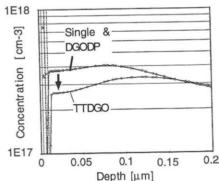
Fig 5. A simulation result of Net concentration profile
