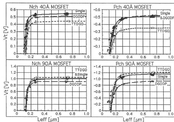
Fig 4.  $V_t$ (Sat) roll-off characteristics
