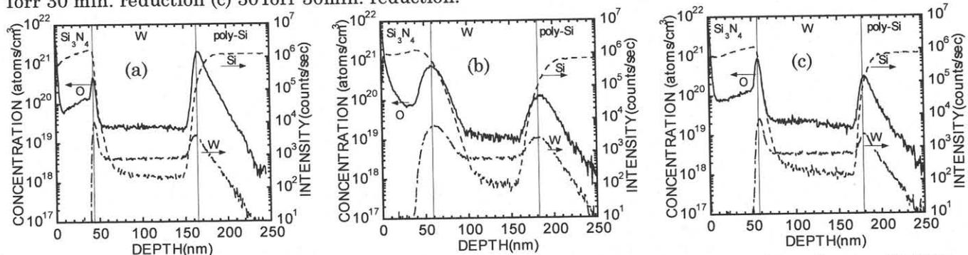
Fig. 7 SIMS profiles of Si<sub>3</sub>N<sub>4</sub> on W with NH<sub>3</sub> in-situ reduction method (a) 0.4Torr 30 min. reduction (b) 30Torr 30 min. reduction (c) ref. 350C load-in, no NH<sub>3</sub> reduction.
