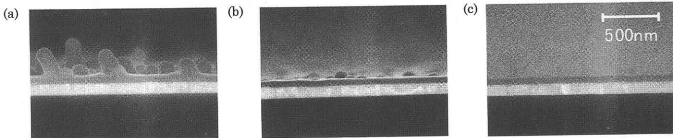
Fig. 5 Surface morphology of low-temperature load-in Si<sub>3</sub>N<sub>4</sub> films on W. (a) 450°C (b) 400°C (c) 350°C
