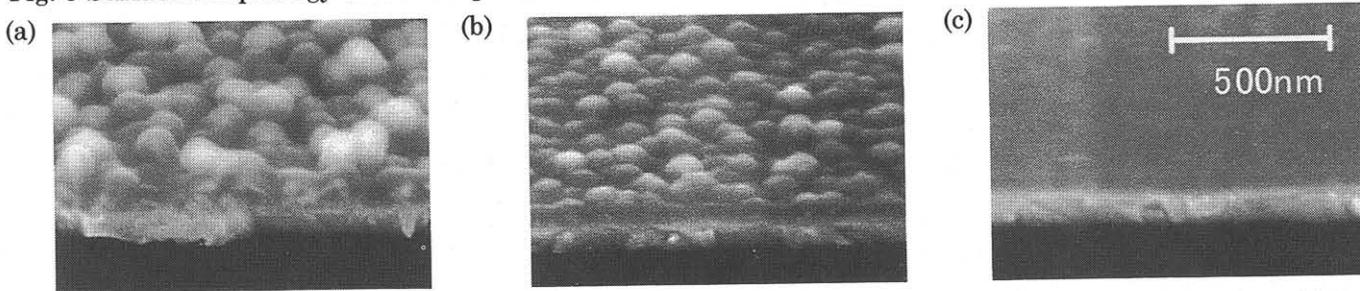
Fig. 6 Surface morphology of Si<sub>3</sub>N<sub>4</sub> surface on W with NH<sub>3</sub> in-situ reduction method. (a) no reduction (b) 0.4 Torr 30 min. reduction (c) 30Torr 30min. reduction.
