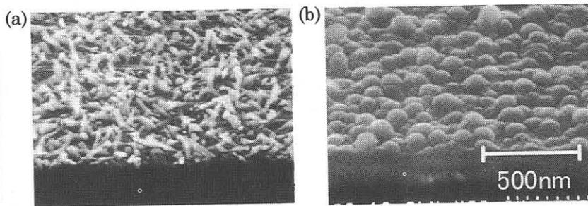
Fig. 4 W surface before (a) and after (b) Si<sub>3</sub>N<sub>4</sub> deposition. Whiskers are observed on W surface before deposition.
