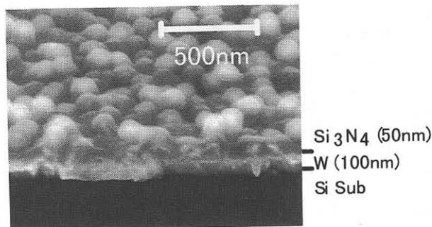
Fig. 2 Abnormal growth of LP-CVD Si<sub>3</sub>N<sub>4</sub> on W.
