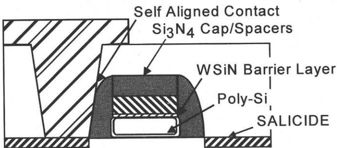
Fig. 1 Concept of self-aligned contact technique of poly-metal with Si<sub>3</sub>N<sub>4</sub> cap/spacers.
