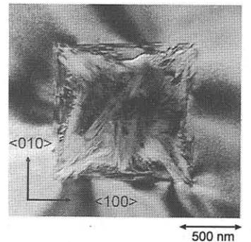
Fig.9 Plane TEM photograph of the mound. The side of the square is parallel to the [110] direction.
