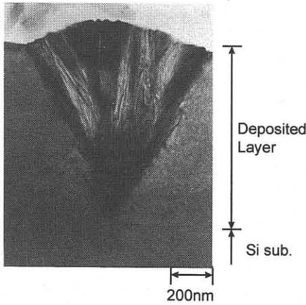
Fig.4 Cross-sectional TEM photograph of the medium-deposition-rate sample, as shown in Fig.2. Mound-shape-defect consists of {111} facets.
