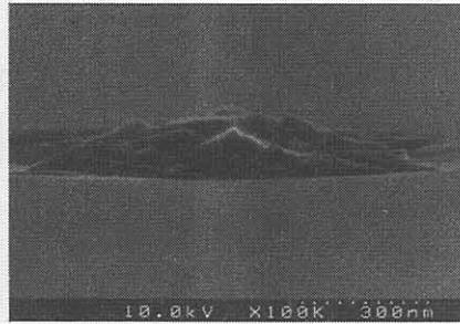
Fig.2 SEM of the Si films deposited under medium deposition rate condition. Total pressure: 10torr, SiH<sub>4</sub>: 900 sccm. Deposition rate: 200nm/min.
