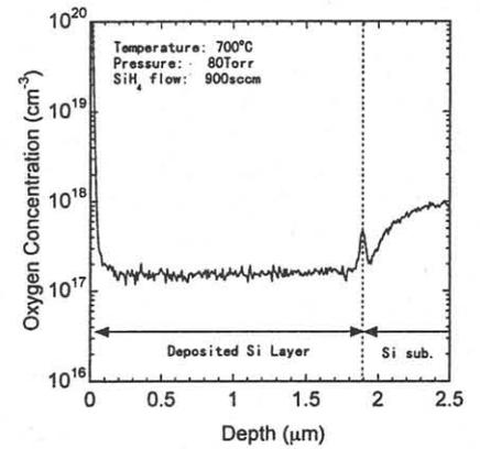
Fig.6 Oxygen profile of the deposited sample, which has a lot of defects in the deposited layer as shown in Fig.3 and 5. The interfacial oxygen concentration was lower than the concentration in the Si substrate.
