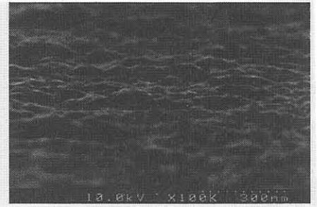
Fig.3 SEM of the Si films deposited under high deposition rate condition. Total pressure: 80torr, SiH<sub>4</sub>: 900 sccm. Deposition rate: 800 nm/min.
