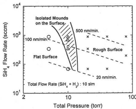
Fig. 8 Surface morphology of the Si films deposited under various conditions. ○, △ and × indicate that the surface of the films was flat, partially rough and rough, respectively. The solid lines show the boundary between the different surface morphology. The broken lines show the deposition rate.
