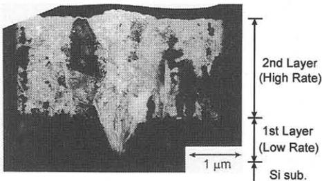
Fig.7 Cross-sectional TEM photograph of the sample, where two Si layers were deposited sequentially. The deposition condition was changed between the 1st and the 2nd layers. High density defects starts not at the surface of the Si substrate but at the interface of the two layers.
