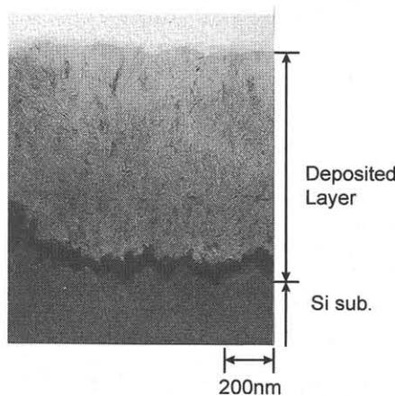
Fig.5 Cross-sectional TEM photograph of the high-deposition-rate sample, as shown in Fig.3. Mound-shape-defects are connected each other, because the density of the defects was very high.
