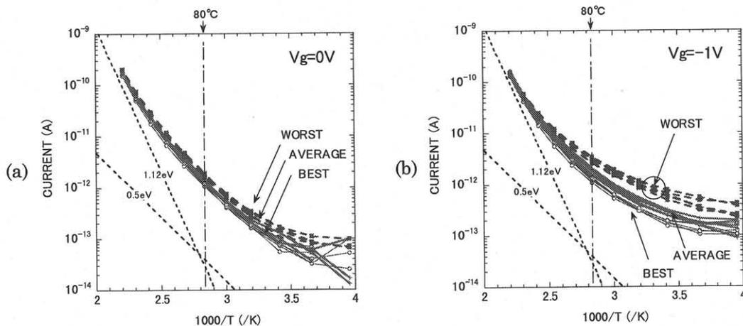
**Figure 3** The leakage dependence on the temperature for each groups, shown in fig.2. Different  $V_g$  was applied,  $V_g=0V$  in fig.3(a), and  $-1V$  in fig3.(b).
