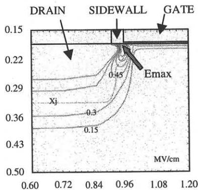
**Figure 4** The simulated profile of the electric field, when negative  $V_g$  was applied.  $V_g=V_{sub}=-1$ .
