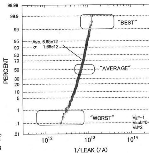
**Figure 2** The typical distribution of leakage current for 490 junctions. 3 groups were extracted for analysis.
