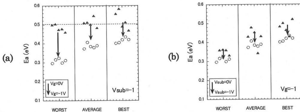
**Figure 5** The activation energy dependence on the bias condition for 3 groups of junctions. The distinctive reduction of  $E_a$  under negative  $V_g$  was observed for 'worst' junctions.
