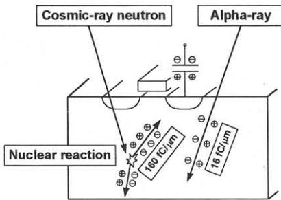
Fig. 1. Alpha and neutron-induced soft error phenomena.
