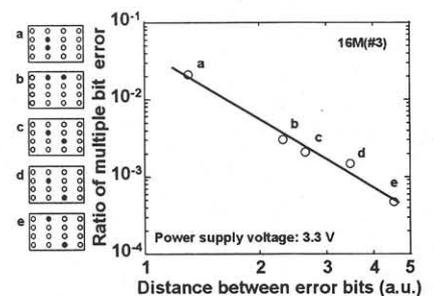
Fig. 5. Ratio of each multiple bit error event vs. the total soft-error events against the distance between the storage nodes in which soft-errors occur.
