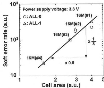
Fig. 3. Soft-error rates for the various unit cell areas.
