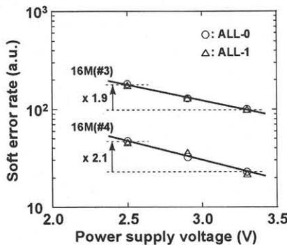
Fig. 4 Soft-error rates as a function of the power supply voltage.
