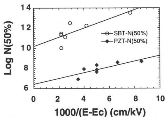
Fig. 5. Electric field strength dependency of the specific switching lifetime ( $N(50\%)$ ).  $N(50\%)$  is the number of switching times when  $Q_{sw}$  decreased to half of the maximum value.  $E_c$  is coercive electric field.
