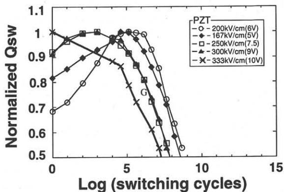
Fig. 2. Changes in normalized switching polarization ( $Q_{sw}$ ) of a PZT capacitor as a function of applied pulse voltage. Definition of  $Q_{sw}$  is described in text.
