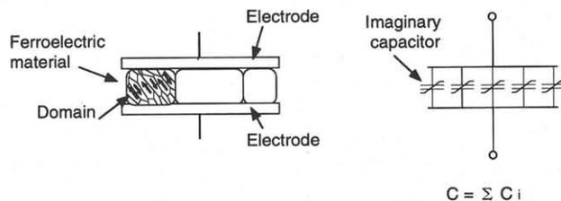
Fig. 4. Actual ferroelectric capacitor (left hand side) and a model capacitor (right hand side). The model capacitor is comprised of imaginary parallel connected capacitors.
