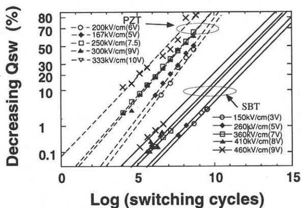
Fig. 3. Log-normal plot of decreasing  $Q_{sw}$ . Solid lines and broken lines are obtained by optimal fitting of data on an SBT capacitor and on a PZT capacitor.
