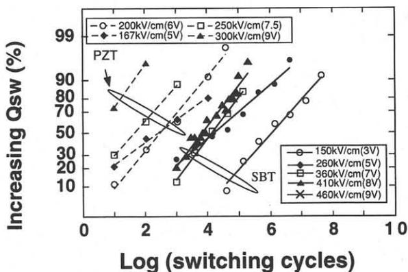
Fig. 6. Log-normal plot of increasing  $Q_{sw}$ . Solid lines and broken lines are obtained by optimal fitting of data on an SBT capacitor and on a PZT capacitor.
