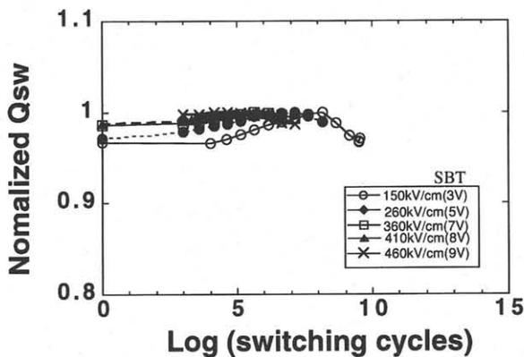
Fig. 1. Changes in normalized switching polarization ( $Q_{sw}$ ) of an SBT capacitor as a function of applied pulse voltage. Definition of  $Q_{sw}$  is described in text.
