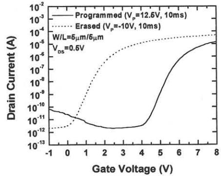
Fig. 3 I<sub>D</sub>-V<sub>G</sub> transfer characteristics of poly-Si TFT EEPROMs after programming and erasing.
