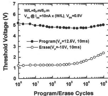
Fig. 5 Endurance characteristics of poly-Si TFT EEPROMs.
