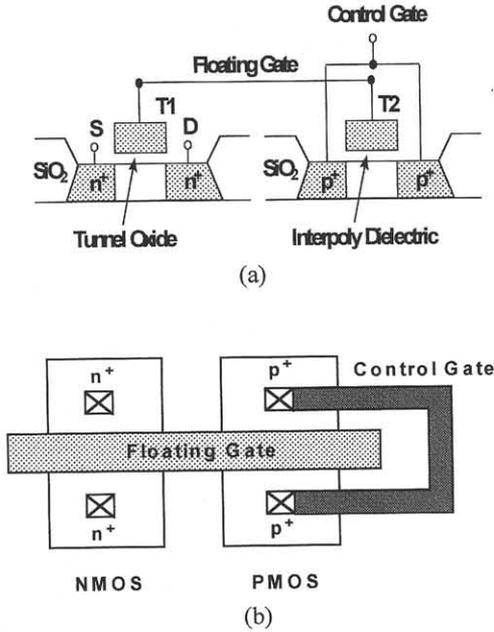
Fig. 1 Cross-sectional (a) and top view (b) of the poly-Si TFT EEPROMs using CMOS poly-Si TFTs with a common floating gate.
