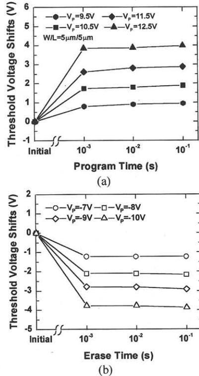
Fig. 4 Programming (a) and erasing (b) characteristics of poly-Si TFT EEPROMs. The programming and erasing were performed through F-N tunneling over the channel area.
