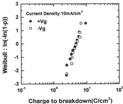
Fig. 2 Weibull plots of charge-to-breakdown of capacitors with ECR N<sub>2</sub>O-plasma oxide under positive and negative constant current density of 10mA/cm<sup>2</sup>.
