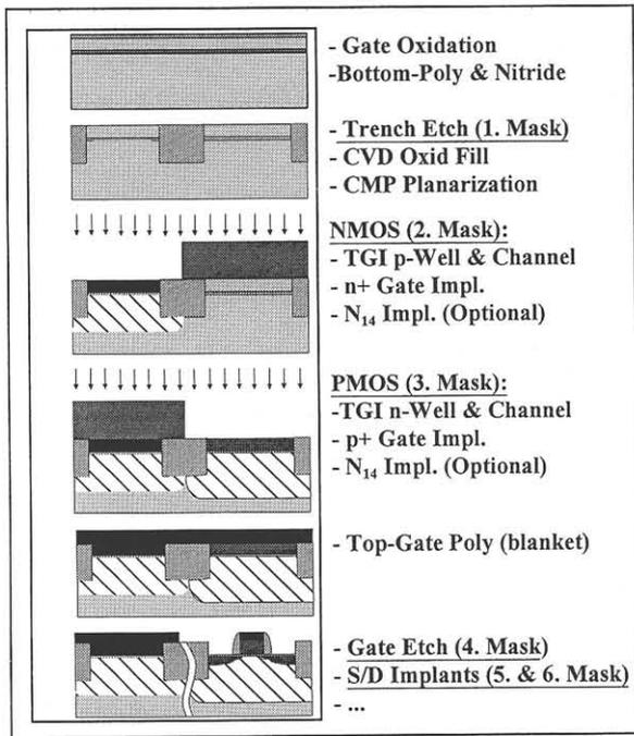
Fig. 1: Essential part of the through-the-gate implanted (TGI) CMOS technology with EXTIGATE [2,3] shallow trench isolation.
