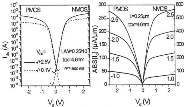
Fig. 3: I-V characteristics obtained by TGI CMOS devices with N<sub>14</sub> co-implantation and EXTIGATE STI isolation.
