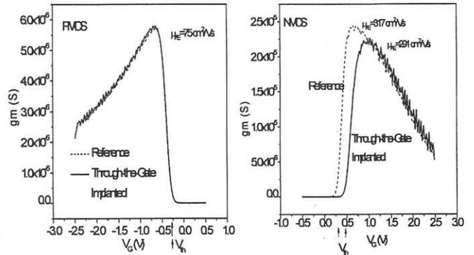
Fig. 4: No mobility loss despite TGI and N<sub>14</sub> implantation.
