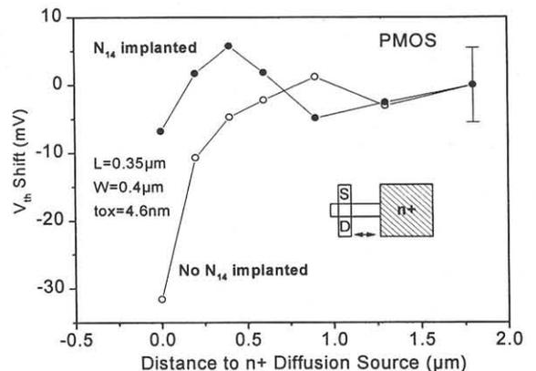
Fig. 7: Counter-doping effects due to lateral impurity diffusion between n+/p+ gates are reduced by N<sub>14</sub> implantation.
