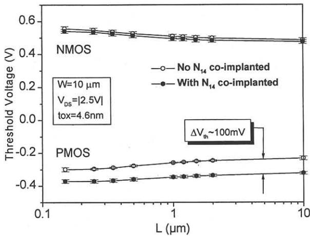
Fig. 2: V<sub>th</sub>(L) characteristics of TGI CMOS with and w/o N<sub>14</sub> co-implantation. V<sub>th</sub> roll-up: 50mV (PMOS) and 70mV (NMOS). Error bars indicate V<sub>th</sub> spread across the wafers.
