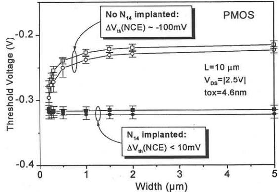
Fig. 5: N<sub>14</sub> co-implantation substantially improves narrow channel effect (NCE) for PMOS devices (2 wafers each split).
