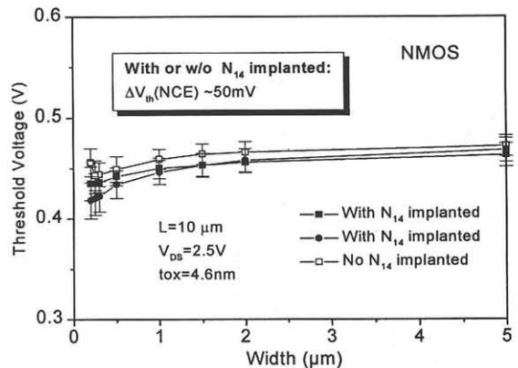
Fig. 6: Narrow channel behavior of NMOS devices is not significantly affected by N<sub>14</sub> co-implantation
