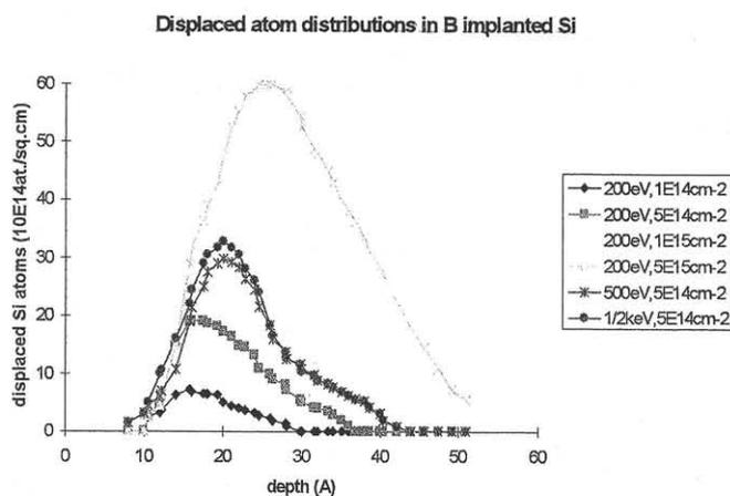
Fig. 1 Displaced atoms in boron implanted silicon measured by MEIS.
