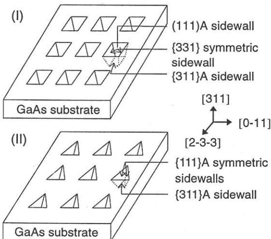
Figs. 1. Schematic illustration of the as-etched GaAs (311)A substrates patterned with (I) square-holes and (II) triangular-holes with acute angle pointing towards  $[-2\bar{3}3]$ .
