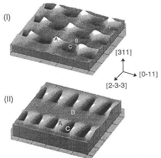
Figs. 2 AFM images of structures I and II. The three portions distinguished by CL are marked A, B and C, respectively.
