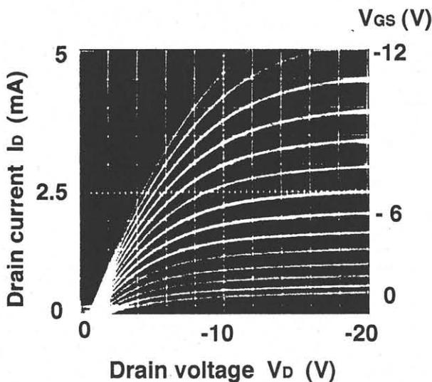
Fig. 2  $I$ - $V$  characteristics of Al/CaF<sub>2</sub>/i-diamond MISFET fabricated by UHV process.
