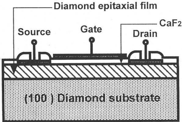
Fig. 1 Schematic view of fabricated MISFET.
