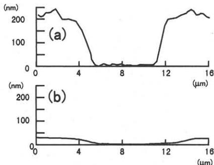
Fig. 4 AFM cross-sectional profiles of the 200-nm-stepped surface (a) before and (b) after being coated with the bottom layer.
