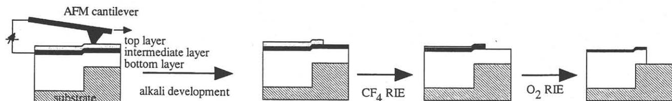
Fig. 1 Process flow of trilayer-resist system using AFM lithography.
