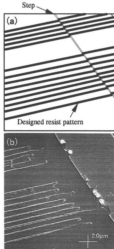
Fig. 3 (a) Designed and (b) formed resist patterns on the 150-nm-stepped surface with a single-layer resist system.
