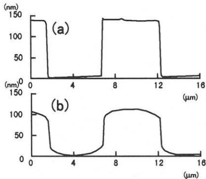
Fig. 2 AFM cross-sectional profiles of the 150-nm-stepped surface (a) before and (b) after being coated with a 40-nm single-layer resist.
