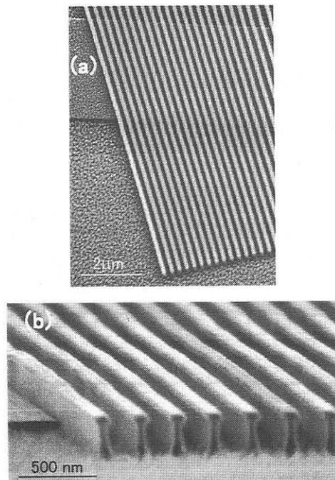
Fig. 5 SEM micrographs of line and space resist pattern fabricated on a 200-nm-stepped surface by a trilayer-resist system.
