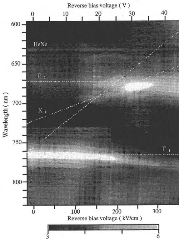
Figure 2: PL spectra as a function of the reverse bias voltage for a laser intensity of 1mW. The brightness is proportional to the logarithm of PL intensity. The intensity range to display the gray level is different in two areas: The top area from 600 - 730 nm shows an approximately  $6 \times 10^{-4}$  intensity range compared to the area of 730 - 830 nm for displaying weak PL. The white dotted lines show the calculated energies which do not take into account the exciton binding energy.
