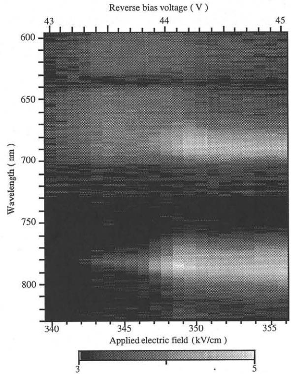
Figure 3: EL spectra as a function of the reverse bias voltage. The brightness is proportional to the logarithm of EL intensity. The intensity range to display the gray level is different in two areas: The top area from 600 - 730 nm shows an approximately  $10^{-1}$  intensity range compared to the area of 730 - 830 nm for displaying a weak EL.
