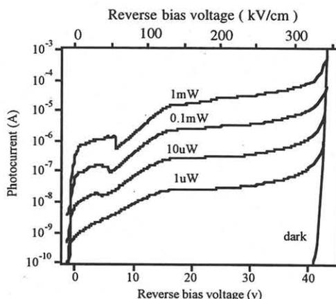
Figure 1: i-V curves at several levels of excitation laser power at 18K.
