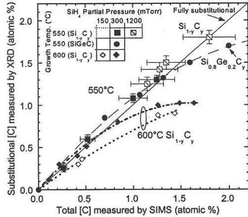
Fig. 4. Comparison of substitutional [C] extracted from XRD to total [C] measured by secondary ion mass spectrometry (SIMS) for  $Si_{1-y}C_y$  and SiGeC epitaxial layers grown by CVD.
