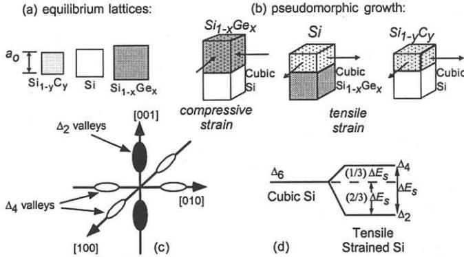
Fig. 1. Schematic (a) equilibrium lattices and (b) pseudomorphic growth. The (c) constant energy diagram and (d) conduction band energy splitting is shown for tensile strained Si.
