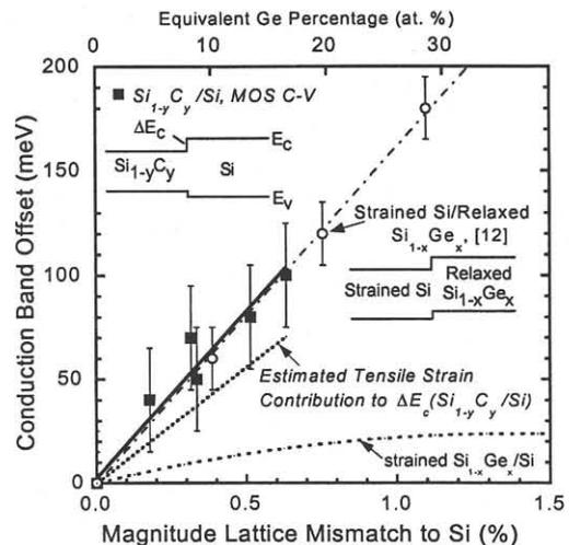
Fig. 6. Conduction band offsets for strained Si/relaxed  $Si_{1-x}Ge_x$  ( $\circ$ ) and  $Si_{1-y}C_y/Si$  ( $\blacksquare$ ), where  $[C]$  (at. %) = mismatch(%)/0.395.
