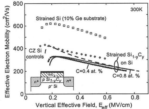
Fig. 5. Measured electron mobilities for strained Si/relaxed  $Si_{1-x}Ge_x$  ( $\square$ ) and  $Si_{1-y}C_y/Si$  (lines)  $n$ -MOSFETs.
