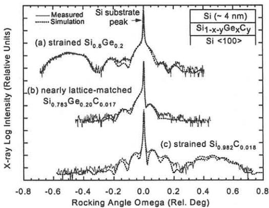
Fig. 3. High resolution XRD (004) rocking curves for (a) 27 nm-thick  $Si_{1-x}Ge_x$ , (b) 24 nm-thick SiGeC, and (c) 22 nm-thick  $Si_{1-y}C_y$  epitaxial layers grown at 550°C by CVD.
