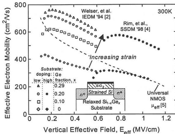
Fig. 2. Measured electron mobilities versus effective field,  $E_{eff} = (Q_{apl} + (1/2) \cdot Q_{inv})/\epsilon$ . Inset shows the strained Si MOSFET structure. The strained Si layer is ~ 10 nm thick.
