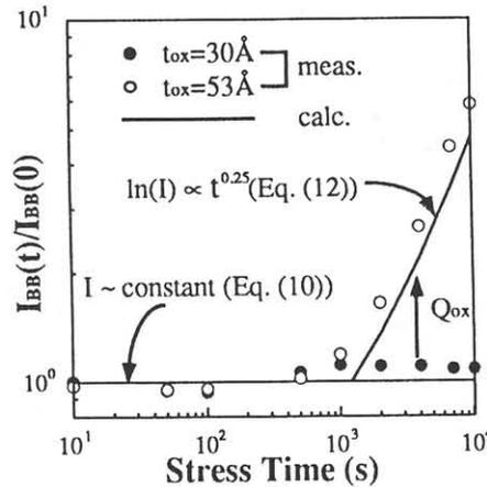
Fig. 4 Stress time dependences of the  $I_{BB}$  measured at  $V_{ds}=1.5V$  and  $V_{gs}=-3.0V$  in 30Å oxide and 53Å oxide n-MOSFET's.
