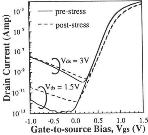
Fig.1 Pre-stress and post-stress  $I_d$ - $V_{gs}$ . Stress time is 3000 sec.
