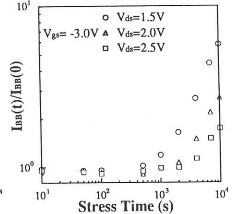
Fig. 5 The  $I_{BB}$  measured at three different biases,  $V_{ds}=1.5V$ ,  $2.0V$ ,  $2.5V$  and  $V_{gs}=-3.0V$  in the 53Å n-MOSFET.
