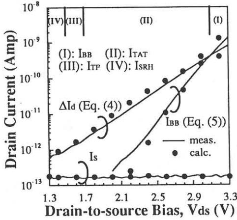
Fig. 2 Various drain leakage current components at  $V_{gs}=0V$ . The dominant drain leakage current in different ranges of  $V_{ds}$  is indicated.
