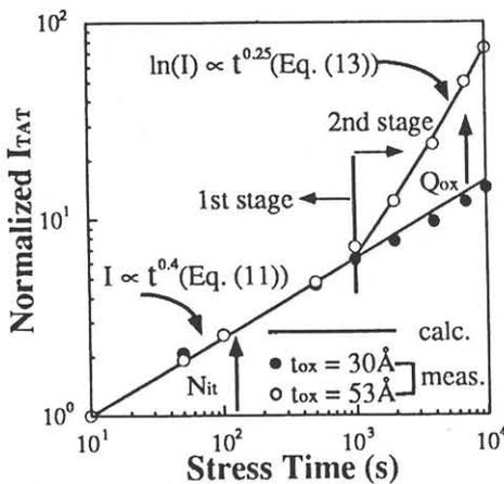
Fig. 3 Stress time dependences of the  $I_{TAT}$  measured at  $V_{ds}=2.5V$  and  $V_{gs}=0V$  in 30Å oxide and 53Å oxide devices. The two  $I_{TAT}$ 's are normalized to have the same initial value.
