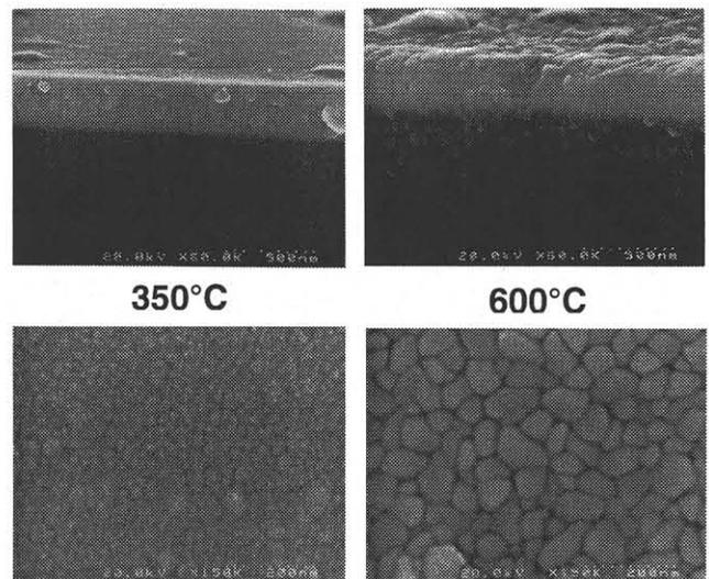
Fig.2 Cross-sectional and surface views of Sr<sub>0.7</sub>Bi<sub>2.8</sub>Ta<sub>2</sub>O<sub>9</sub> on SiO<sub>2</sub>/n-Si(100) diode structure as a parameter of substrate temperature
