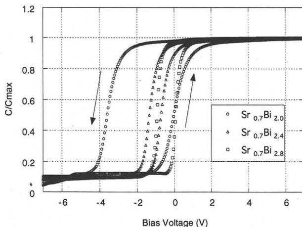
Fig.5 C-V characteristics of Al/Sr<sub>0.7</sub>Bi<sub>2+x</sub>Ta<sub>2</sub>O<sub>9</sub>/SiO<sub>2</sub>/n-Si(100) diode structure as a function of x (=0.8,0.4,0) in laser ablation deposition (measured frequency: 1MHz)
