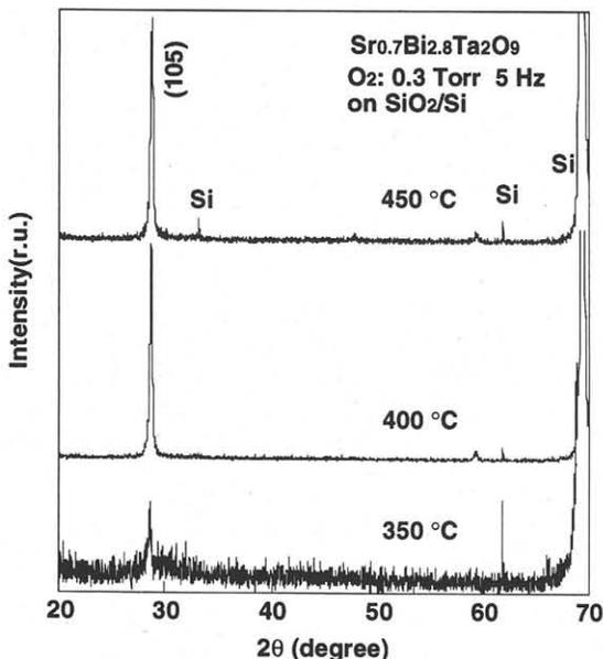
Fig.1 XRD patterns of Sr<sub>0.7</sub>Bi<sub>2.8</sub>Ta<sub>2</sub>O<sub>9</sub> films on SiO<sub>2</sub>/Si wafers as a function of substrate temperature
