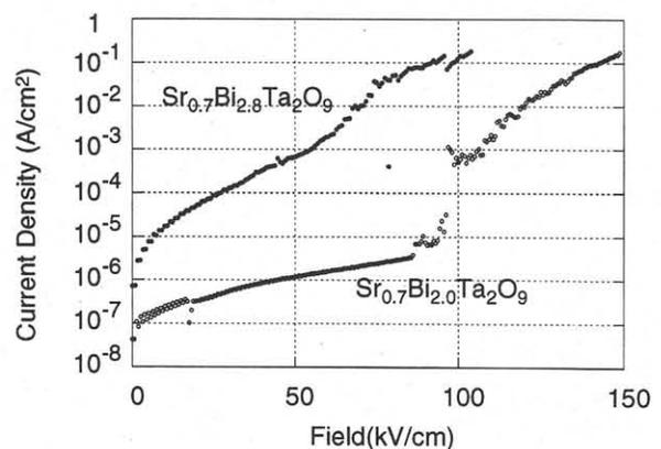
Fig.3 Current density vs. electric field for Al/Sr<sub>0.7</sub>Bi<sub>2+x</sub>Ta<sub>2</sub>O<sub>9</sub>/SiO<sub>2</sub>/n-Si(100) diode structure when forward biased as a parameter of x (=0.8,0) in laser ablation deposition
