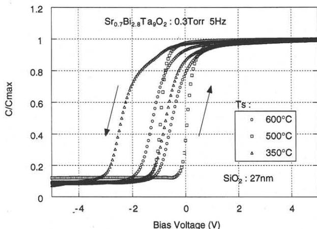
Fig.4 C-V characteristics of Al/Sr<sub>0.7</sub>Bi<sub>2.8</sub>Ta<sub>2</sub>O<sub>9</sub>/SiO<sub>2</sub>/n-Si(100) diode structure as a function of substrate temperature in laser ablation deposition (measured frequency: 1MHz)
