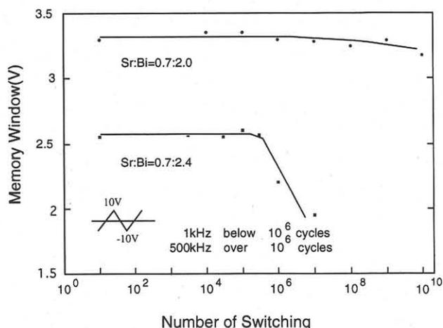
Fig.6 Fatigue characteristics of memory window in C-V curve in MFIS diode structure for Sr/Bi of 0.7/2.0 and 0.7/2.4
