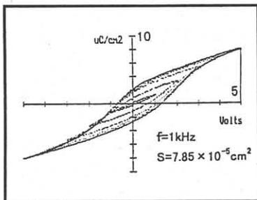
Fig.5 D-E hysteresis loops of non-annealed 100nm- $\text{Bi}_4\text{Ti}_3\text{O}_{12}$ .
