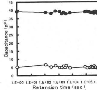
Fig.9 Retention property of Pt/100nm- $\text{Bi}_4\text{Ti}_3\text{O}_{12}$ /30nm $\text{Bi}_2\text{SiO}_5$ /Si/Al.
