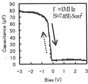
Fig.3 C-V characteristics of Pt/30nm $\text{Bi}_2\text{SiO}_5$ /Si/Al.
