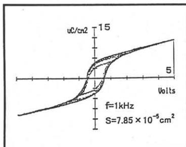
Fig.7 D-E hysteresis loops of annealed 100nm- $\text{Bi}_4\text{Ti}_3\text{O}_{12}$ .
