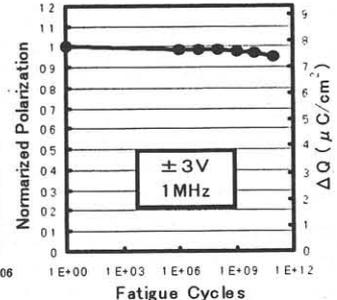
Fig.10 Fatigue property of 100nm- $\text{Bi}_4\text{Ti}_3\text{O}_{12}$ .
