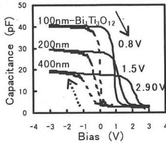
Fig.4 C-V characteristics of Pt/ $\text{Bi}_4\text{Ti}_3\text{O}_{12}$ /30nm $\text{Bi}_2\text{SiO}_5$ /Si/Al.
