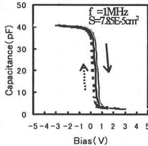
Fig.6 C-V characteristics of non-annealed 100nm- $\text{Bi}_4\text{Ti}_3\text{O}_{12}$ .
