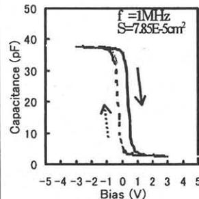
Fig.8 C-V characteristics of annealed 100nm- $\text{Bi}_4\text{Ti}_3\text{O}_{12}$ .
