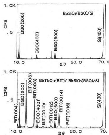
Fig.1 XRD patterns of  $\text{Bi}_2\text{SiO}_5/\text{Si}$  and  $\text{Bi}_4\text{Ti}_3\text{O}_{12}/\text{Bi}_2\text{SiO}_5/\text{Si}$ .
