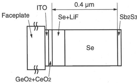
Fig. 3. Cross section of the a-Se HARP film.
