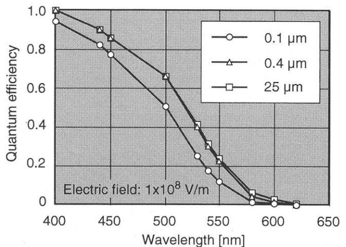
Fig. 2. Dependence of quantum efficiency on the a-Se thickness and wavelength.
