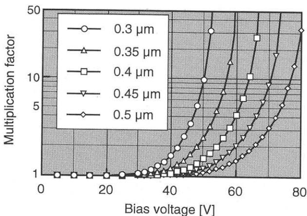
Fig. 1. Dependence of multiplication factors on the a-Se thickness and bias voltage.
