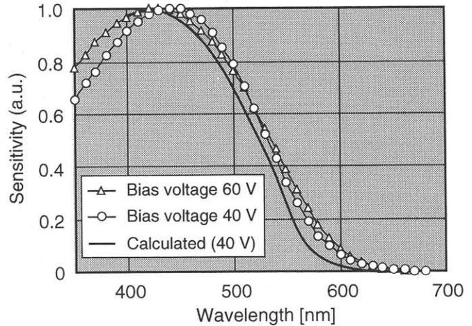
Fig. 4. Spectral response of the a-Se HARP film.
