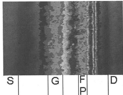
Fig. 4. Spatial distribution of electroluminescence from FPFET biased at  $V_{ds}=20\text{V}$  and at  $V_{gs}=-0.1\text{V}$ .
