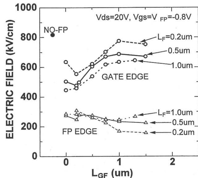
Fig. 3. Peak Electric field at gate and FP edges as a function of  $L_{GF}$  for FPFETs ( $L_F=0.2, 0.5, 1.0\mu\text{m}$ ) biased at  $V_{ds}=20\text{V}$ . Peak electric field at the gate for MESFET (NO-FP) is also shown.
