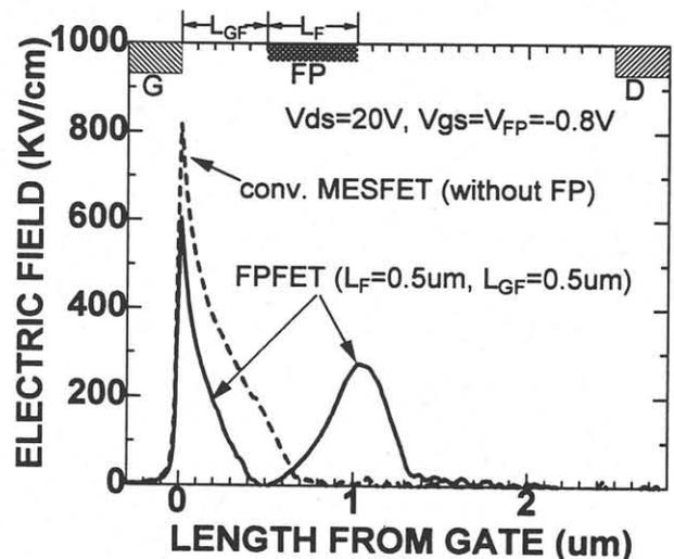
Fig. 2. Electric field distributions in the channel for conventional MESFET and FPFET biased at  $V_{DS}=20\text{V}$  and at  $V_{GS}(=V_{FP})=-0.8\text{V}$ .
