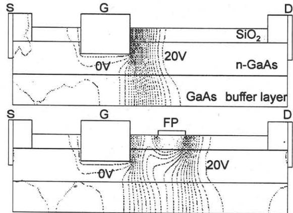
Fig. 1. Potential distributions for conventional MESFET (upper) and FPFET (lower) biased at  $V_{DS}=20\text{V}$  and at  $V_{GS}(=V_{FP})=-0.8\text{V}$ .
