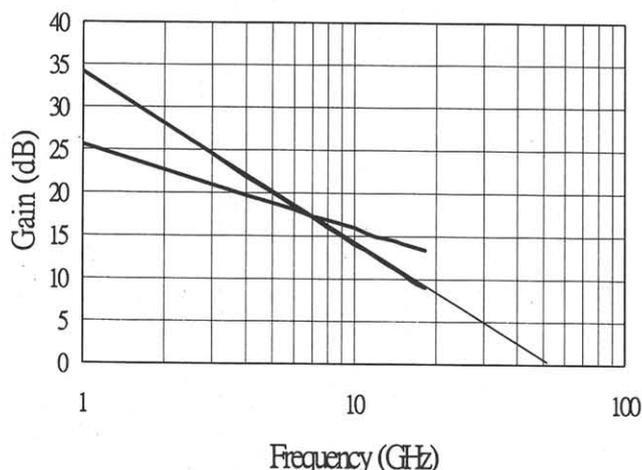
**Fig. 3.** Gain versus frequency for a typical 1.1- $\mu\text{m}$   $\text{In}_{0.52}\text{Al}_{0.48}\text{As}/\text{InAs}/\text{In}_x\text{Al}_{1-x}\text{As}$  pseudomorphic HEMT with multiple  $\text{InAs}/\text{In}_{0.52}\text{Al}_{0.48}\text{As}$  monolayer superlattices buffer.
