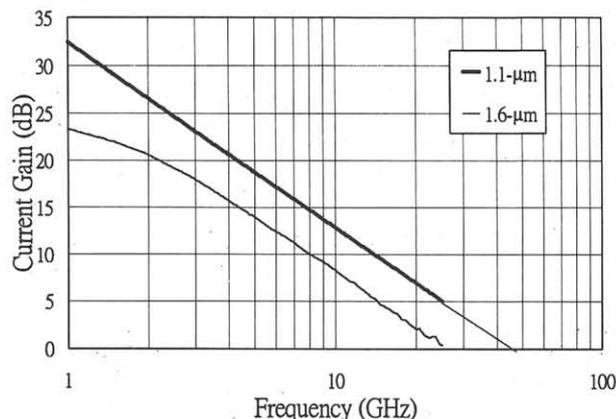
**Fig. 4.** Gain versus frequency for 1.1- $\mu\text{m}$  and 1.6- $\mu\text{m}$   $\text{In}_{0.80}\text{Ga}_{0.20}\text{As}/\text{In}_{0.25}\text{Ga}_{0.75}\text{As}$  pseudomorphic HEMT's.
