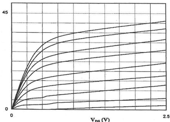
**Fig. 2.** I-V characteristics of a typical 1.1- $\mu\text{m}$   $\text{In}_{0.52}\text{Al}_{0.48}\text{As}/\text{InAs}/\text{In}_x\text{Al}_{1-x}\text{As}$  pseudomorphic HEMT with multiple  $\text{InAs}/\text{In}_{0.52}\text{Al}_{0.48}\text{As}$  monolayer superlattices buffer ( $V_{\text{GS}}=-0.2$  V/step, 0.4 V top curve).
