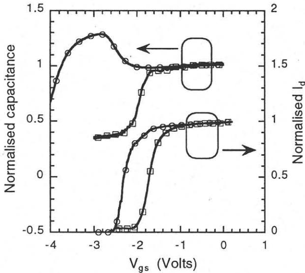
Fig. 3. Normalised capacitance and drain current characteristics for large area devices with (circles) and without (squares) nanodots.
