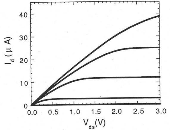
Fig. 2. MISFET transistor characteristics for a large area device without nanodots at room temperature.
