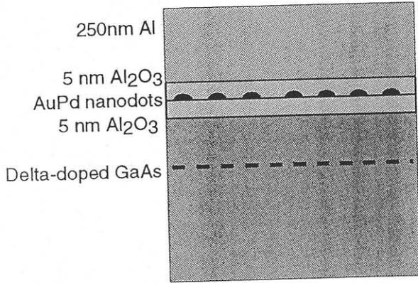
Fig. 1. Schematic cross-sectional diagram of the nanocomposite gate  $\delta$ -doped GaAs MISFET structure.
