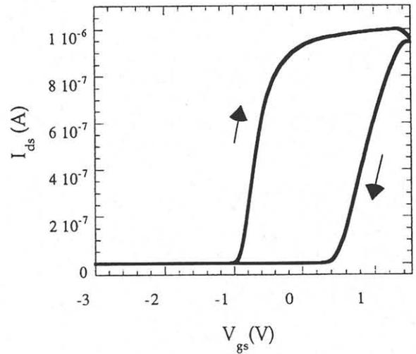
Fig. 4. Drain current hysteresis for a wide channel device measured at 77K. The gate voltage is swept between -3V and 1V in the directions indicated by the arrows.
