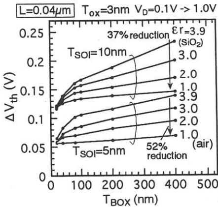
Fig.3  $\Delta V_{th}$  dependence on  $T_{BOX}$ .
