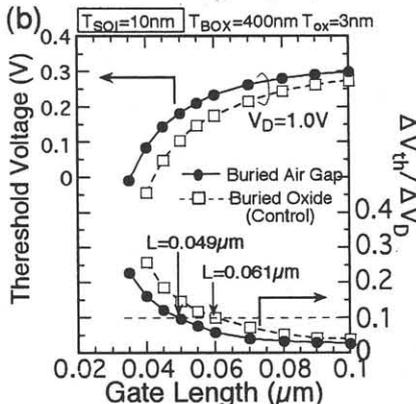
Fig.6  $V_{th}$  dependence on  $L$
