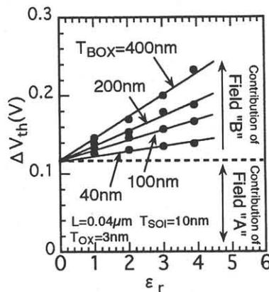
Fig.4  $\Delta V_{th}$  dependence on  $\epsilon_r$ .
