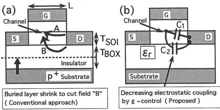
Fig.1 Buried layer Engineering. Arrow "A" represents the drain field through the SOI layer, and "B" through the buried layer. Capacitance  $C_1$  and  $C_2$  the electrostatic coupling corresponding to "A" and "B", respectively.
