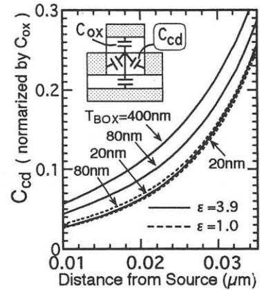
Fig.5 The Capacitance between the drain and the channel.
