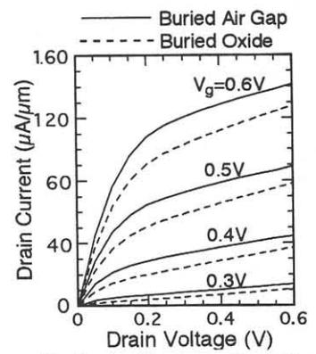
Fig.9  $I_D$ - $V_D$  characteristics.
