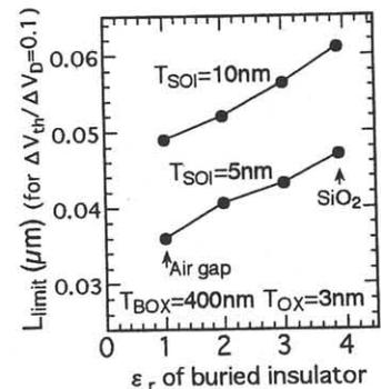
Fig.8 DIBL limit dependence on the buried layer structure.
