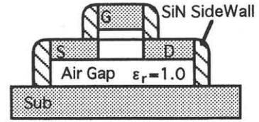
Fig.2 A possible buried low  $\epsilon$  layer structure. The buried oxide of conventional SOI wafer is removed by wet etching after forming S/D. A porous  $\text{SiO}_2$  buried layer in the bonded wafer is also considered to be possible.
