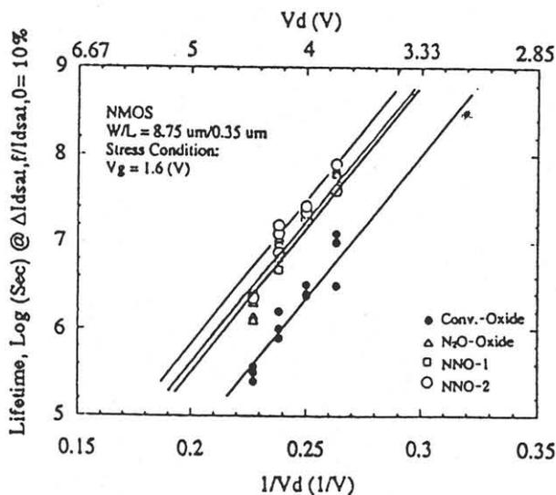
Fig.3. Extracted lifetimes of NMOS devices with 55 Å different gate dielectrics
