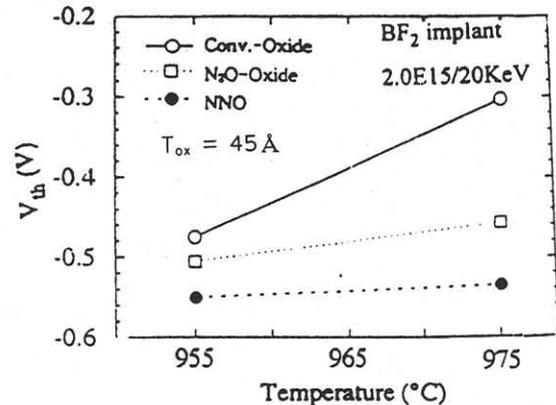
Fig.4. Shift in threshold voltage of PMOS devices
