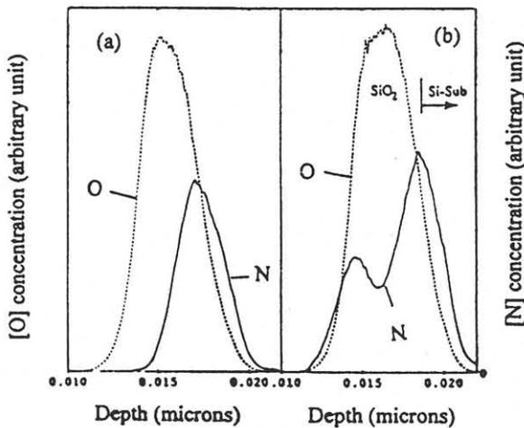
Fig.1 SIMS depth profiles for 85Å nitrided gate dielectrics: (a) N<sub>2</sub>O-Oxide and (b) NNO samples
