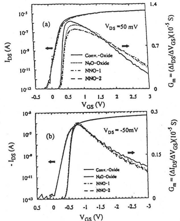
Fig.2. Drain current and transconductance characteristics for 55 Å gate dielectrics: (a) NMOS and (b) PMOS devices ( $W/L = 40\mu m/40\mu m$ )
