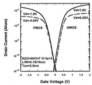
Fig.9 Subthreshold characteristics
