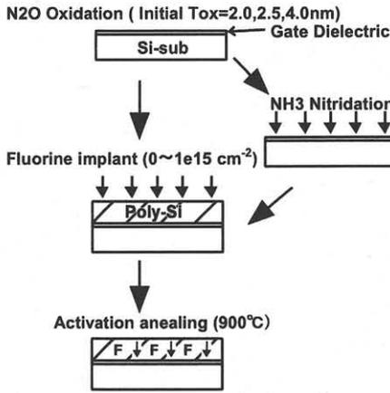
Fig.1 procedure of gate dielectrics formation
