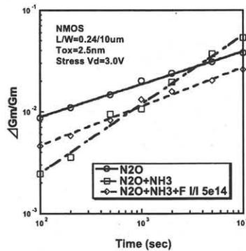
Fig.11 Time dependence of Gm degradation in NMOS
