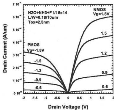
Fig.10 Id-Vd characteristics
