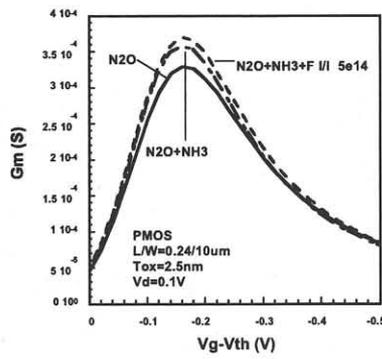
Fig.8 Gm vs (Vg-Vth) characteristics of PMOS
