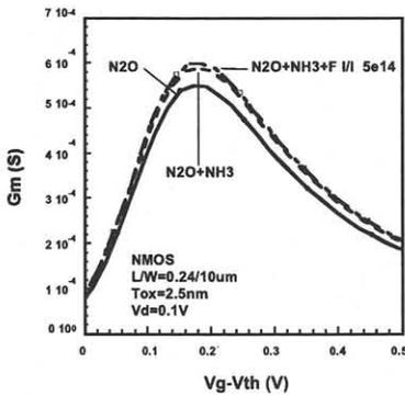
Fig.7 Gm vs (Vg-Vth) characteristics of NMOS
