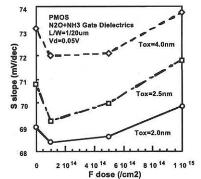
Fig.6 Fluorine dose dependence of S-slope
