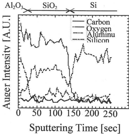
Fig.1 AES depth profile of Al<sub>2</sub>O<sub>3</sub>/Si with O<sub>2</sub> anneal.
