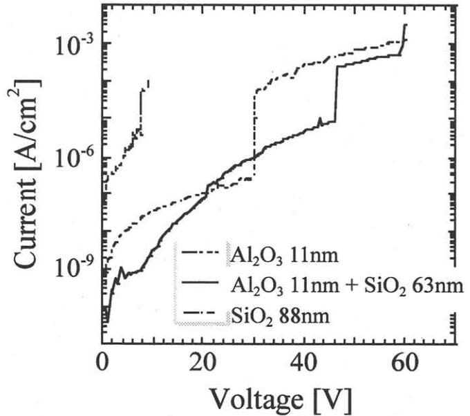
Fig.2. Properties of brake-down voltages of various insulator/Si samples.
