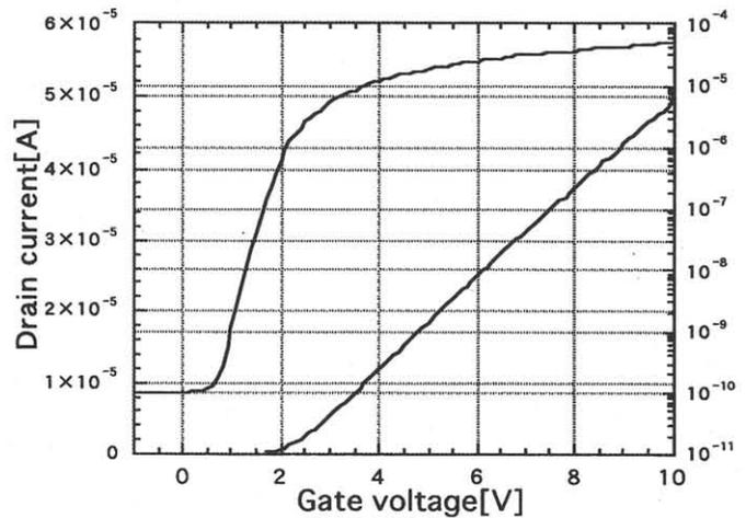
Fig.4. I<sub>D</sub>-V<sub>G</sub> of nMOS FET on SOI.
