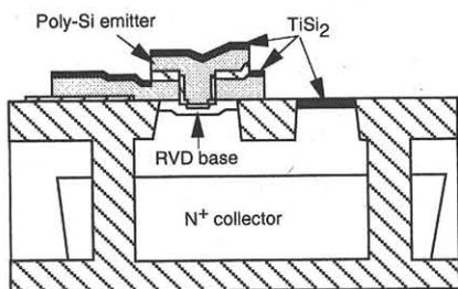
Fig. 1 Transistor cross section.
