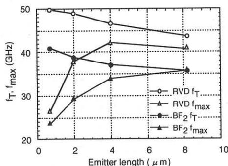
Fig. 7  $f_T, f_{max}$  vs.  $L_E$
