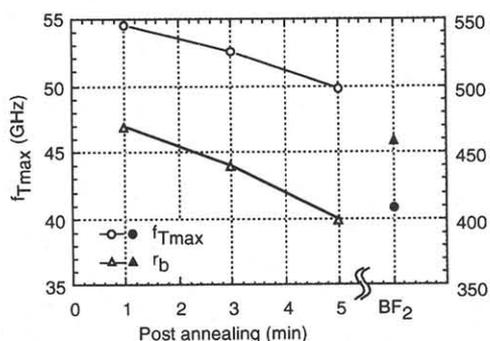
Fig. 6  $f_{Tmax}$  and  $r_b$ .
