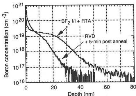
Fig. 3 Boron profiles in base region.
