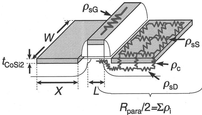
Fig. 1. Schematic diagram of parasitic resistance of salicided MOSFET and physical lengths significant for electrical properties.
