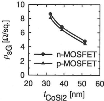
Fig. 2(a). Dependence of sheet resistivity of gate electrodes on silicide thickness.
