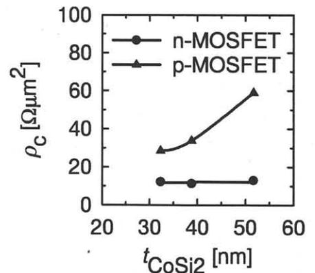
Fig. 3(a). Dependence of specific contact resistivity of CoSi<sub>2</sub>/Si interface on silicide thickness.
