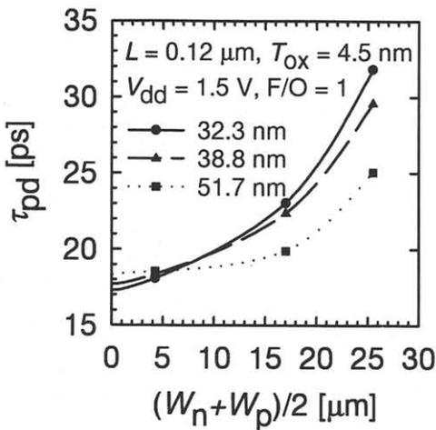
Fig. 4. CMOS propagation delay vs. channel width for three different thickness of silicide layer. In larger  $W$  region,  $\tau_{\text{pd}}$  is improved with increasing silicide thickness, while, in smaller  $W$  region,  $\tau_{\text{pd}}$  is degraded due to increase of contact resistance.
