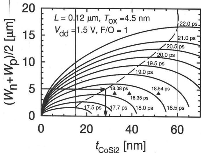
Fig. 5. Contour line of  $\tau_{\text{pd,tot}}$  on  $t_{\text{CoSi}_2}$ - $W$  plane for CMOS inverter ( $F/O=1$ ). Symbols show measured data. Dashed line indicates optimized combination of channel width and  $t_{\text{CoSi}_2}$ . Once channel width is determined,  $t_{\text{CoSi}_2}$  should be selected on dotted line.
