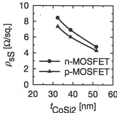
Fig. 2(b). Dependence of sheet resistivity of source/drain electrodes on silicide thickness.
