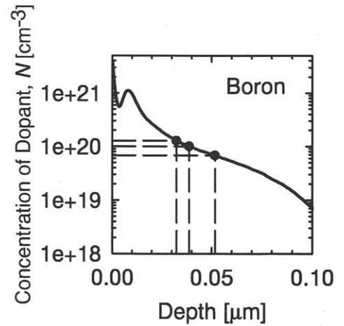
Fig. 3(b). Depth profile of Boron atoms by SIMS. Closed circles indicate CoSi<sub>2</sub>/Si interfaces. Dashed lines indicate  $t_{\text{CoSi}_2}$ , silicide thickness, and corresponding  $N$ , dopant concentration.
